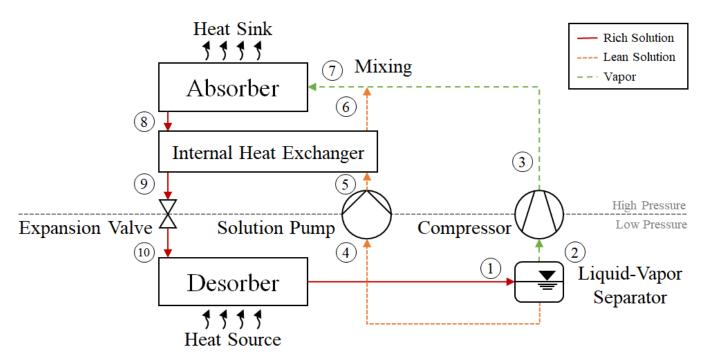
Figure 1. Schematic representation of a basic hybrid absorption-compression heat pump cycle.
