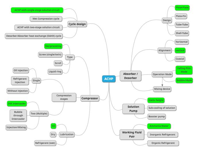
**Figure 6.** Overview of recent developments and existing solutions for the realization of ACHP systems (fields highlighted in green indicate the currently most frequently used solutions for commercial applications of each system part).
