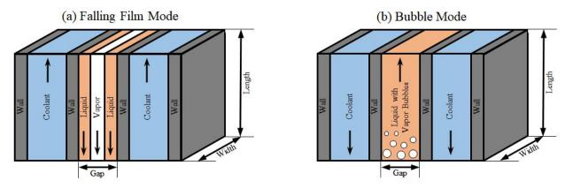
**Figure 5.** Schematic representation of a plate heat exchanger operated as absorber in (**a**) falling film and (**b**) bubble mode (adapted from Ahrens et al. (2019) [75]).
