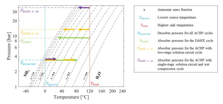
Figure 3. Simplified comparison of the described ACHP cycles in a ln p-1/T diagram (adapted from Groll (1997) [18]).
