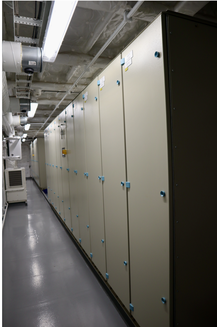
Figure 5.8: One of the four batteries on board MF Lagatun
