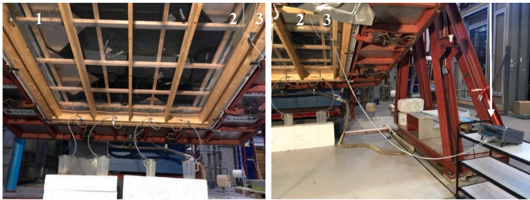
Fig. 13. Raintightness test setup in the laboratory. The set of 3 tubes to measure air pressure difference are marked. Tube 1 for measuring the differential air pressure by the RAWI box, and tubes 2 and 3 for measuring the differential air pressure connected to the external micromanometer. Study 3 (Table 3).
