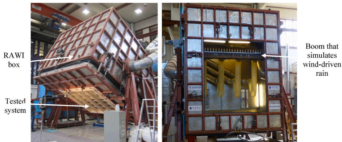
Fig. 1. Large-scale turnable box for rain and wind tightness testing of sloping building surfaces (RAWI box), while test is running (left) [20] and RAWI box without a test sample (right) [21]. Schematic drawing of RAWI box is shown in Fig. 12.
