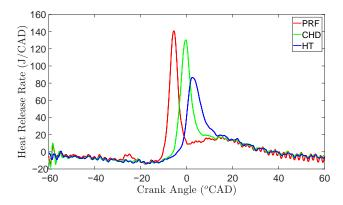
Figure 10. Heat release rate for the three fuels with T<sub>inlet</sub> 115 °C.
