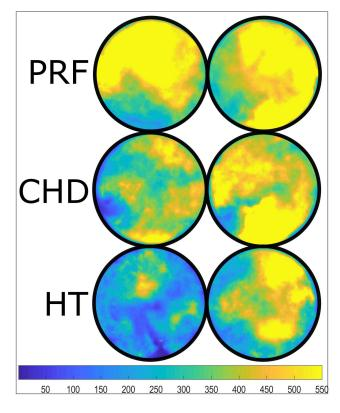
**Figure 14.** Sample images from a combustion cycle. Images shown are for each fuel, at the two  $T_{inlet}$  considered ( $T_{inlet}$  90 °C (**left**),  $T_{inlet}$  115 °C (**right**)). Contrast adjusted so all flame is visible (very low intensity flame shown as light blue). The images are taken from one cycle at the CAD where peak pressure for that condition was achieved.
