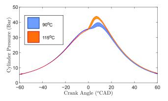
**Figure 11.** Combustion pressure for HT at  $T_{inlet}$  90 °C (blue) and 115 °C (red). Solid region indicates the range of combustion pressures collected. Plotted as an alternative to plotting all 8 combustion pressures as individual curves.
