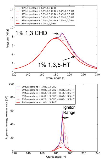
**Figure 2.** Chemical kinetic engine simulation of a 1% 1,3-cyclohexadiene (1,3-CHD) in 99% n-pentane converted in various fractions to 1,3,5-hexatriene (1,3,5-HT). The cylinder pressure (**upper graph**) and apparent heat release rate (**lower graph**) show that a concentration of 1% is effective in controlling ignition photo-chemically in the engine.
