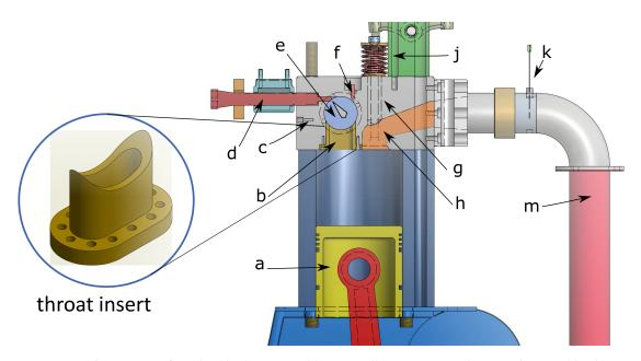
**Figure 4.** OACIC in place on top of single cylinder engine (**a**). Piston; (**b**). Connecting throat and insert; (**c**). Thermocouple; (**d**). Injector; (**e**). Optically accessible combustion region; (**f**). Pressure transducer; (**g**). Valves (**h**). Inlet and outlet; (**j**). Valve rocker arms; (**k**). Inlet pressure transducer and temperature thermocouple; (**m**). Inlet heater. Throat insert shown in detail.
