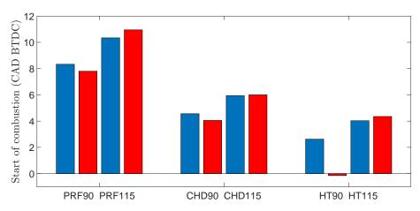
**Figure 13.** Start of combustion determined from combustion pressure (blue) and optically (red) for the three fuels at the two  $T_{inlet}$  considered.
