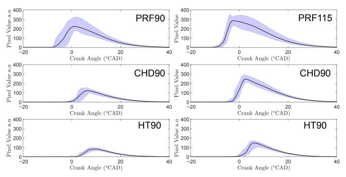
**Figure 12.** Average pixel intensity (arbitrary units a.u) collected by high speed camera against CAD. Solid black line is the mean value from 8 combustion events, the blue region around the line indicates the range.
