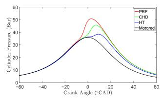
Figure 7. Combustion pressure for the three fuels and motored pressure with T<sub>inlet</sub> 90 °C.
