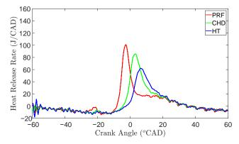
Figure 8. Heat release rate for the three fuels with T<sub>inlet</sub> 90 °C.
