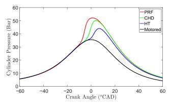
Figure 9. Combustion pressure for the three fuels and motored pressure with T<sub>inlet</sub> 115 °C.
