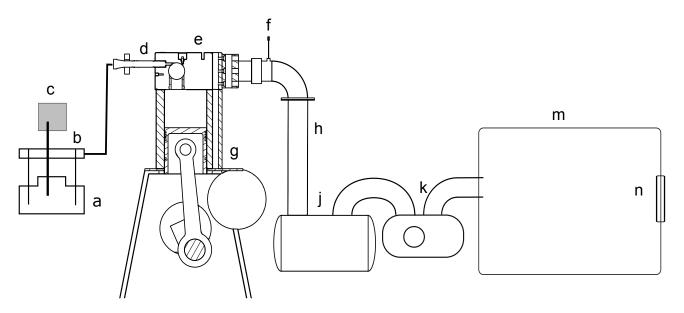
**Figure 5.** (a) High pressure pump; (b) Common rail; (c) Fuel tank; (d) Injector; (e) OACIC; (f) Inlet thermocouple and pressure transducer; (g) Engine; (h) Heater; (j) Settling tank; (k) Roots compressor; (m) Airbox; (n) Orifice plate.
