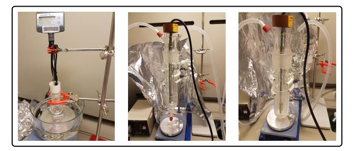
**Figure 3.** Reactors used. (**Left**)—roundbottom flask with Pen-Ray lamp inserted, in water bath. (**Center**)—immersion well reactor. (**Right**)—the configuration of the reactor resulted in limited space available for the stirrer magnets, therefore the reactor flask was modified with the bottom tap of the reactor removed.
