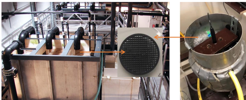
Fig. 5. Semi-commercial MBBR at Nofima Sunndalsøra (left), photo: Nofima. Small-scale reactors (right), photo: R. Fossmark. The biocarriers (centre) are AnoxK™ Chip P (Krüger Kaldnes AS, Norway).
