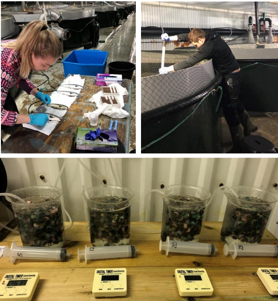
Fig. 4. Anette Bugten sampling faeces from the fish for microbial analysis (top left) and Kristian Nordøy netting fish for sampling (top right). Capacity stress-tests of biofilter carriers with different salinities (bottom). Photos: R.O. Fossmark.
