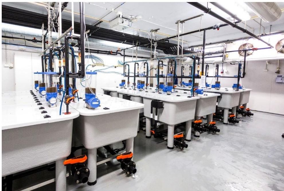
Fig. 3. Research facility at NTNU Sealab. This picture shows the fish hall. 12 of the tanks are connected to two (6 fish tanks each) and separate RAS water treatment loops (in a separate room) and were used in this study. Photo: Sintef Ocean
