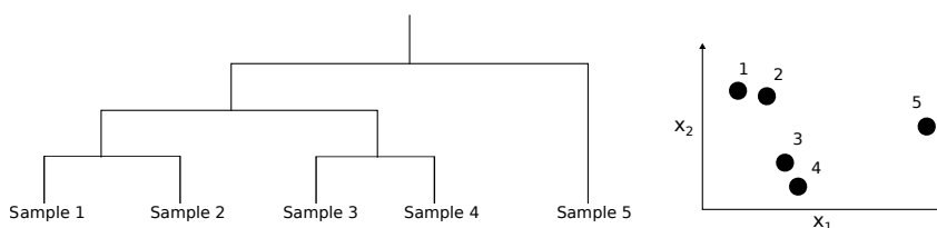
Figure 4.5: Illustration of agglomerative clustering in a two-dimensional input space. The tree to the left illustrates the distance structure for the points to the right, with sample 1 and 2, and 3 and 4 being closest.
