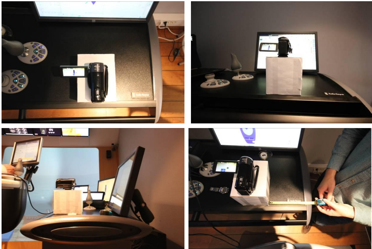
Figure 12. Set-up of the camera that captures the position and heading footprint screen
