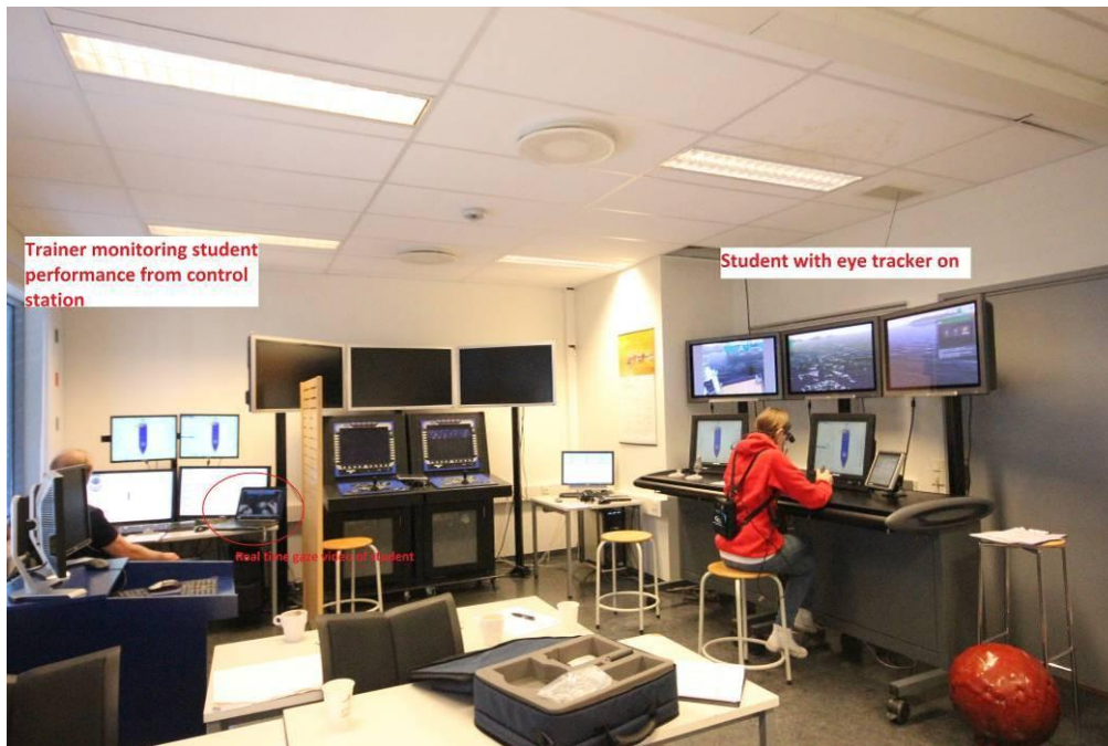
Figure 5. Experimental setup of DP training, from previous study [23]
