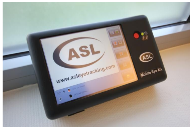
Figure 37. ASL eye-tracker Display/Transmit Unit DTU
