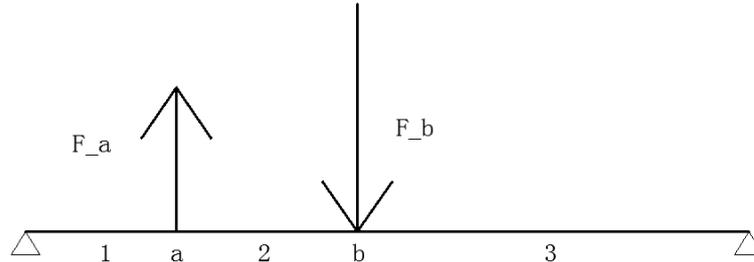
**Figure 3-15 Divide the beam into 3 parts**
