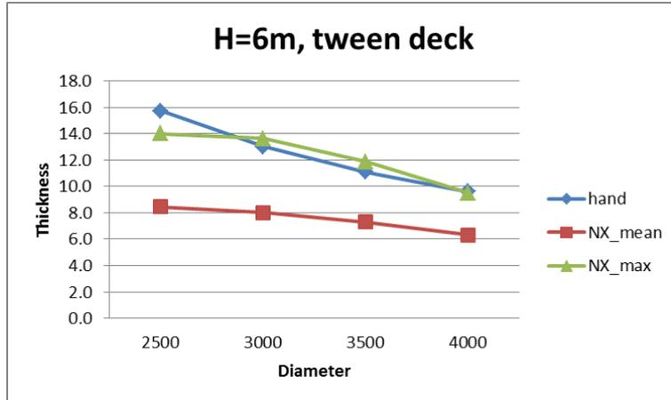
Figure 0-11 Thicknesses of tween deck of varying diameters when penetrating to 3 decks
