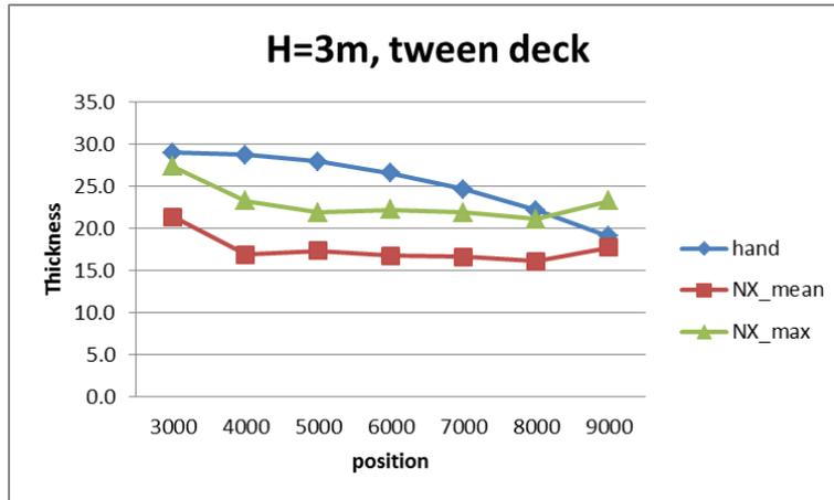
Figure 0-2 Thicknesses of tween deck of varying positions when penetrating to 2 decks
