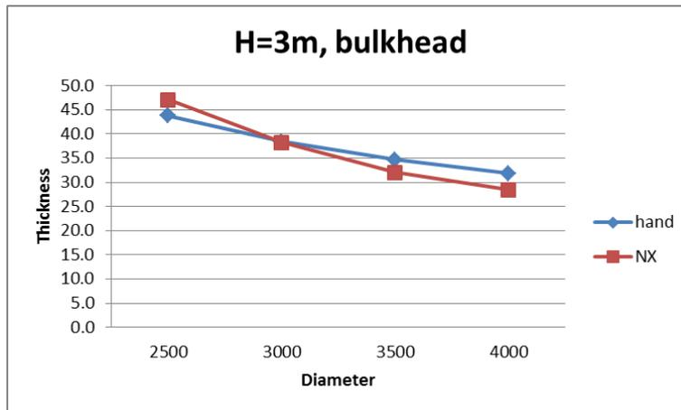
**Figure 0-6 Thicknesses of bulkhead of varying diameters when penetrating to 2 decks**
