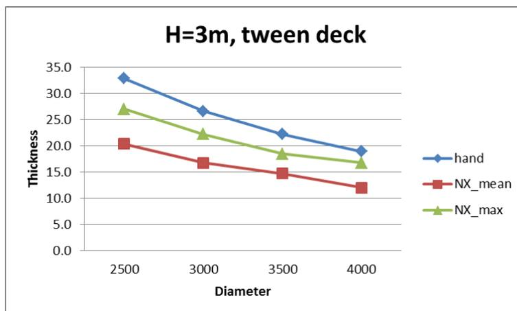
**Figure 0-5 Thicknesses of tween deck of varying diameters when penetrating to 2 decks**
