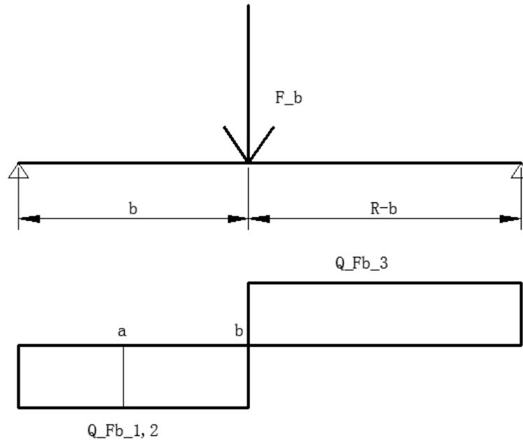
**Figure 4-11 Shear force of  $F_b$**
