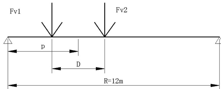
**Figure 3-12 Design vertical force  $F_v$**
