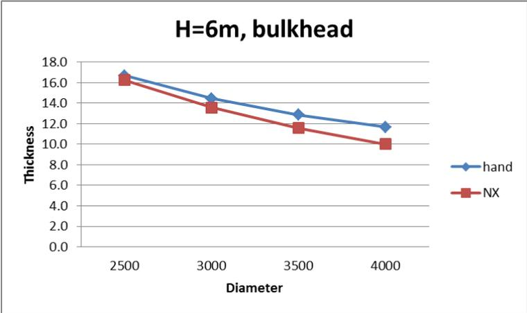
Figure 0-12 Thicknesses of bulkhead of varying diameters when penetrating to 3 decks
