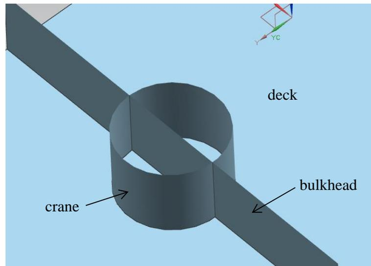
**Figure 3-2 Cut-open view of the structure**
