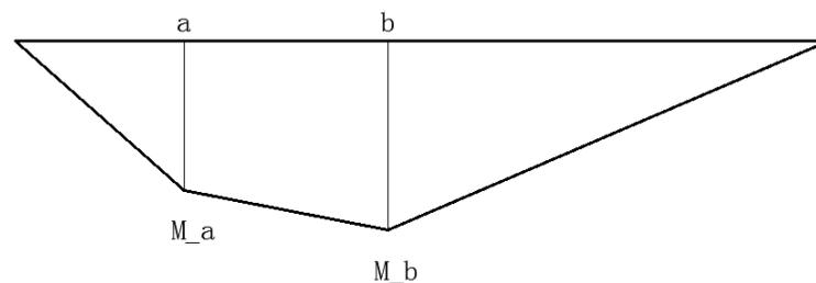
**Figure 4-15 Combined bending moment of Fv1 and Fv2**
