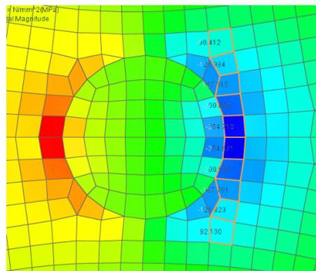
**Figure 6-1 Elements used for calculating stress**
