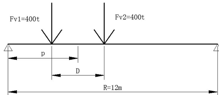
**Figure 4-12 Load condition of  $F_v$**
