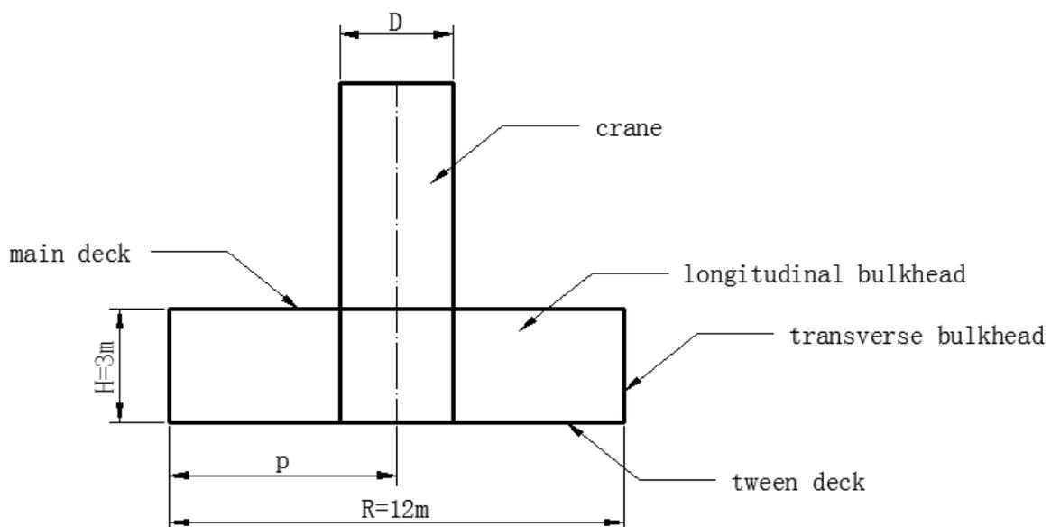
Figure 1-3 Crane penetrating into two decks
