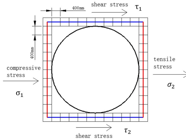
**Figure 3-8 Elements checked for calculating stress**
