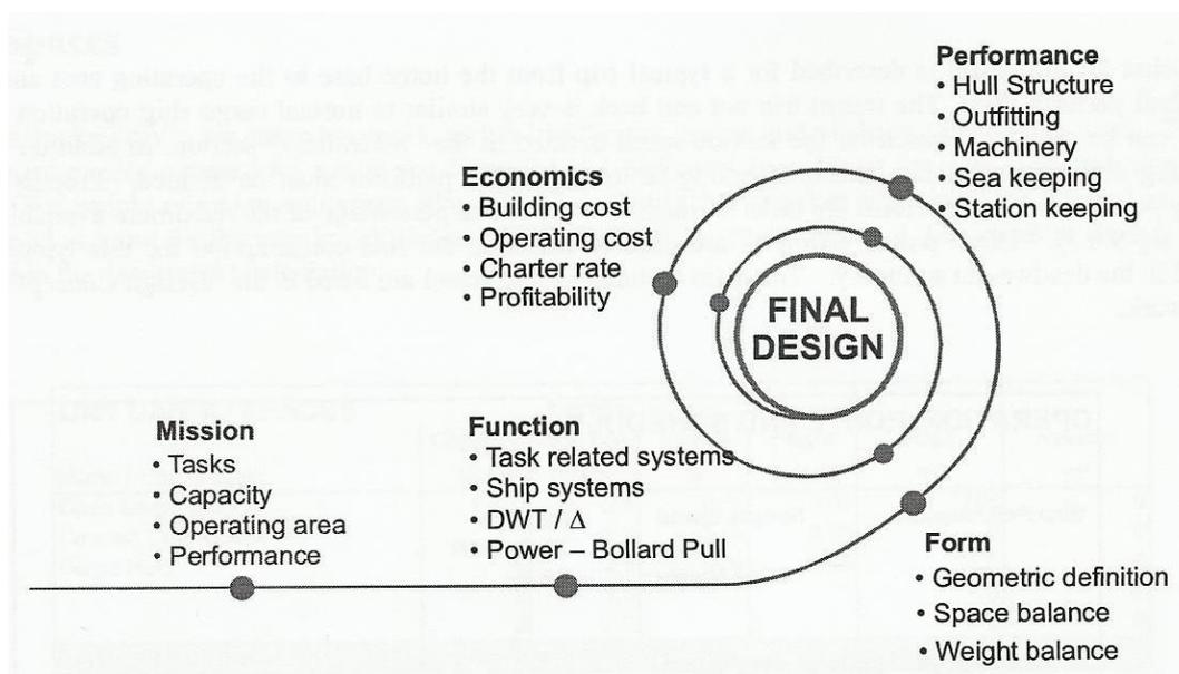
Figure 1-2 Offshore vessel design process
