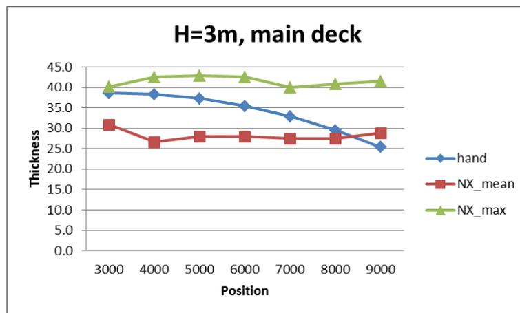
**Figure 0-1 Thicknesses of main deck of varying positions when penetrating to 2 decks**
