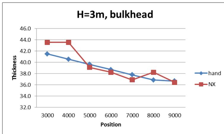
Figure 0-3 Thicknesses of bulkhead of varying positions when penetrating to 2 decks
