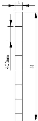
**Figure 3-11 Cross section area of bulkhead**
