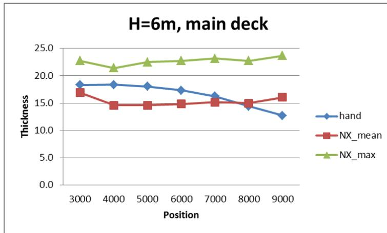
Figure 0-7 Thicknesses of main deck of varying positions when penetrating to 3 decks
