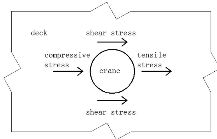
Figure 3-6 Stress allocation on deck
