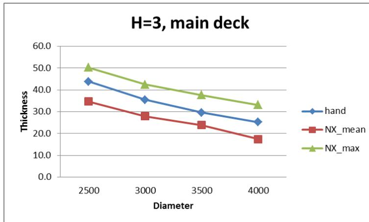
**Figure 0-4 Thicknesses of main deck of varying diameters when penetrating to 2 decks**
