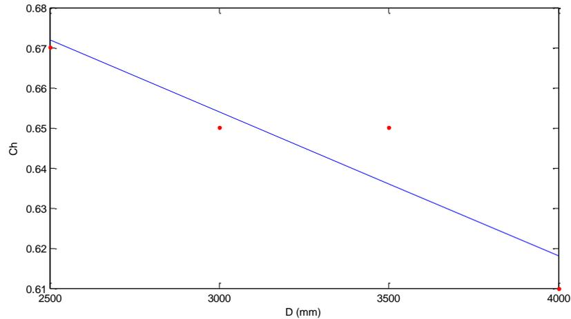
**Figure 4-2 Ch for varying diameters when H=3m**
