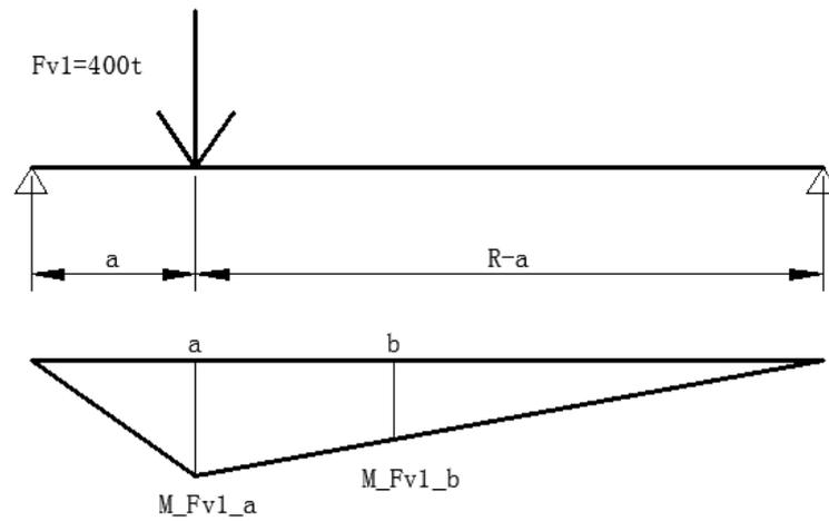
**Figure 4-13 Bending moment for Fv1**
