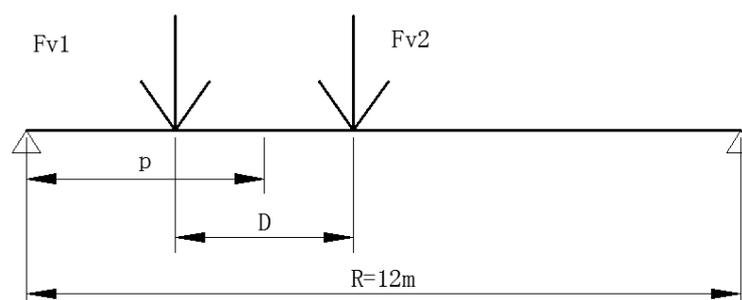
**Figure 4-6 Design vertical force  $F_v$**
