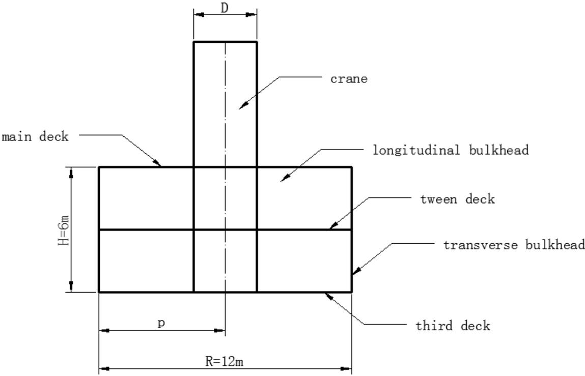
Figure 1-4 crane penetrating into three decks
