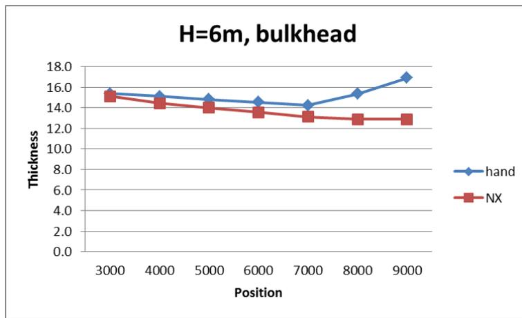
**Figure 0-9 Thicknesses of bulkhead of varying positions when penetrating to 3 decks**
