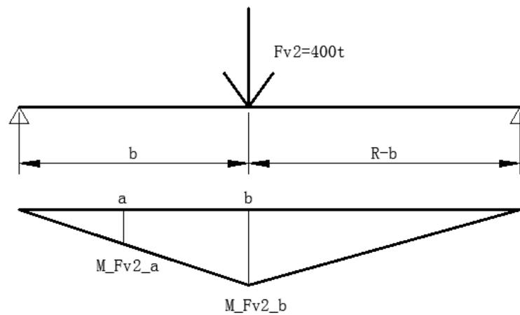
**Figure 4-14 Bending moment for Fv2**
