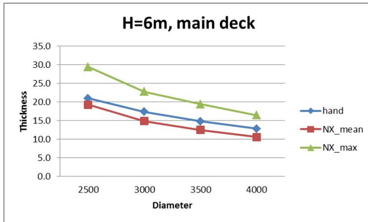
Figure 0-10 Thicknesses of main deck of varying diameters when penetrating to 3 decks
