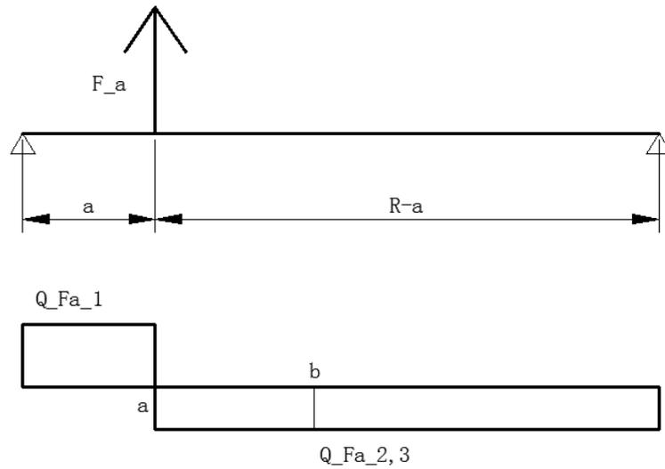
**Figure 4-10 Shear force of  $F_a$**
