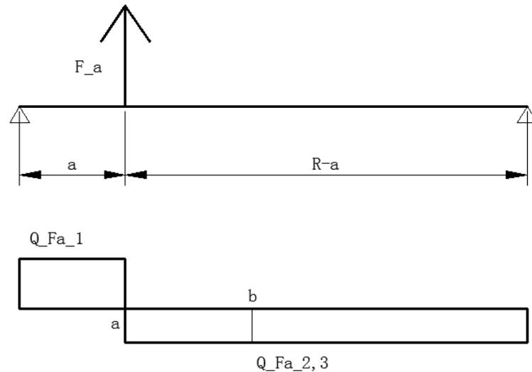
**Figure 3-16 Shear force of Fa**
