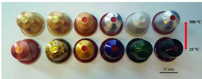
**Fig. 18.** Different coffee capsules before and after holding at 500 °C for 3 h [23].
