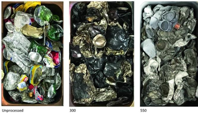
**Fig. 16.** Effect of de-coating temperature. From left unprocessed material, de-coating at 300 and 550 °C [22].
