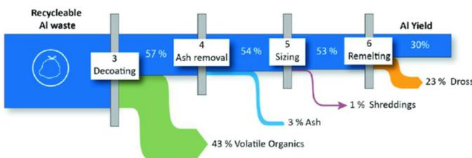
Fig. 15. Recycling process steps for Al-recovery [22].
