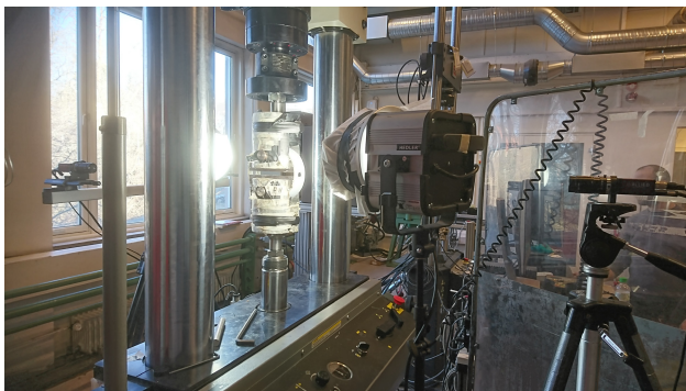
Figure 3: Split disk setup with composite ring installed. Cameras on each side and strong lights to provide enough light for the short shutter speed.
