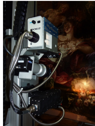
(b) Vertically-mounted push-broom hyperspectral system with motorized XY axes scanning a painting.
