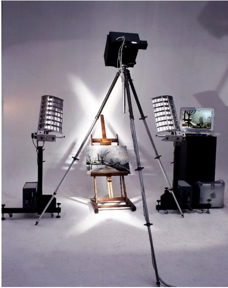
Figure 2.6: 13 filter portable multispectral CRISATEL camera. (Image source: [38])
