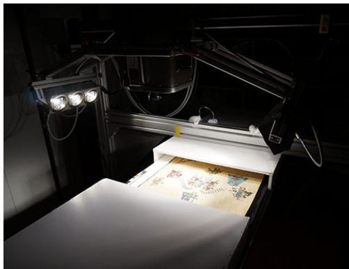
(a) Horizontally-mounted push-broom hyperspectral system with motorized Y-axis scanning a manuscript.
