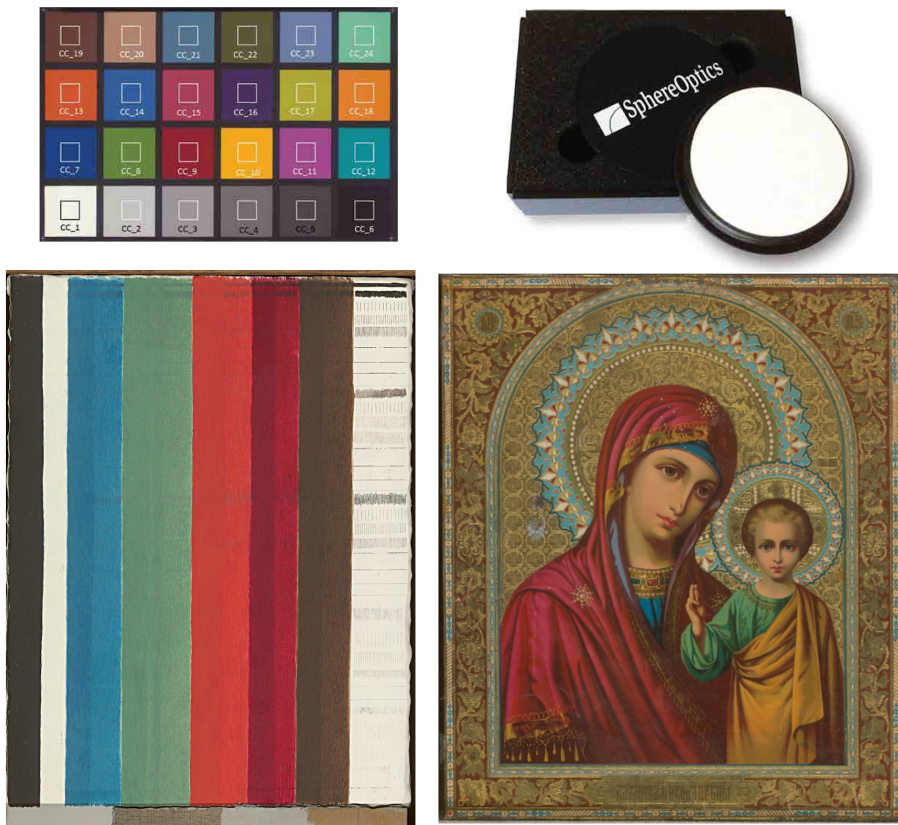
Figure 2.10: Targets used in the spectral imaging round-robin test: 24 patch Macbeth ColorChecker (top left), wavelength standard featuring well-defined and narrow features over the UV, visible and near infra-red spectral ranges (top right), custom-made pigment panel with 7 Renaissance-era pigments (bottom left) and a mass-produced 19 th century Russian icon made through polychrome lithography (bottom right). (Image source: [8])
