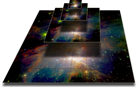
Figure 3: Illustration of tiled multi-resolution pyramid with 4 levels of resolution.
