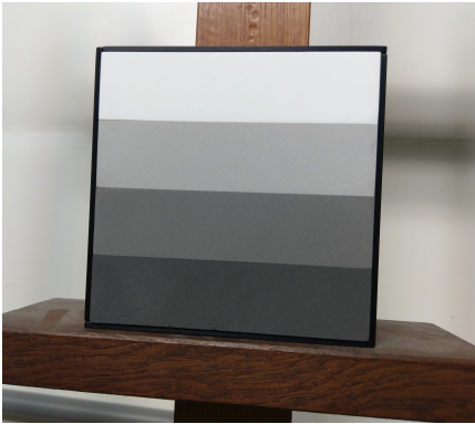
Figure 2. Multi-step reflectance standard with reflectances at 99%, 50%, 25% and 12.5%
