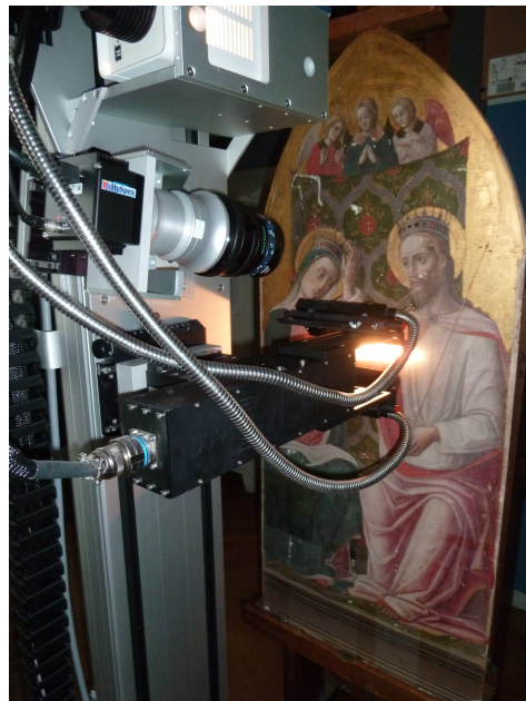
Figure 2.7: Hyperspectral imaging system at the C2RMF, Paris: 160-band pushbroom camera with wavelength range of 400–1000 nm mounted on XY translation stage
