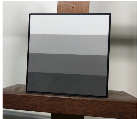
Figure 2.11: Multi-step reflectance standard with reflectances at 99%, 50%, 25% and 12.5%
