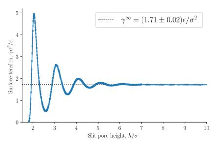
**Figure 8.** Surface tension  $\gamma$  as a function of slit pore height h, see Equation (33). The dashed line shows the surface tension at infinite separation  $\gamma^{\infty}$ .
