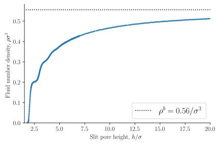
**Figure 3.** Fluid number density  $\rho = N/V$  as a function of slit pore height h. The bulk fluid number density is shown as a dashed line.
