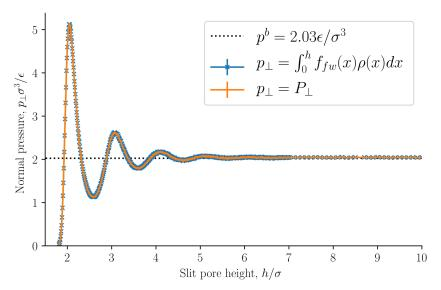
**Figure 7.** Normal pressure  $p_{\perp} = P_{\perp}$  as a function of slit pore height h. It is computed as the normal mechanical pressure tensor component, see Equation (31), and as the integral of the fluid–solid force times the local fluid density, see Equation (32).
