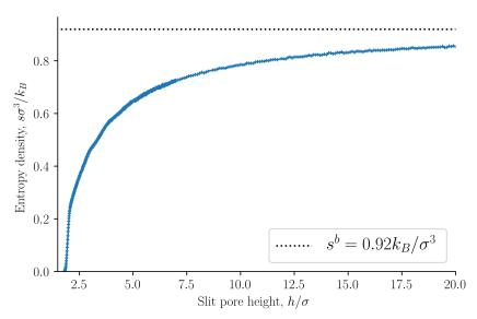
**Figure 4.** Entropy density s = S/V as a function of slit pore height h. See Equation (36). The dashed line shows the entropy density of the bulk  $s^b$ .
