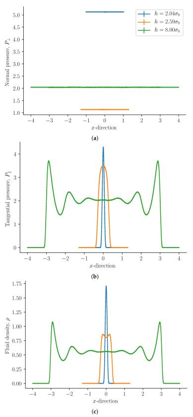
**Figure 2.** (a) Normal mechanical pressure, (b) tangential mechanical pressure, and (c) fluid number density  $\rho$  as a function of the x-direction for slit pore heights  $h = 2.04\sigma$ ,  $2.59\sigma$ , and  $8\sigma$ .
