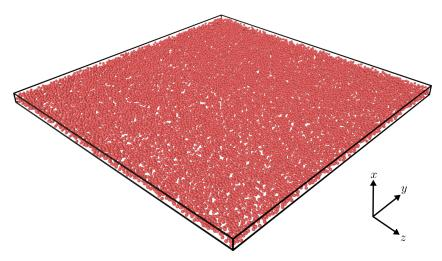
**Figure 1.** Visualization of the fluid particles in a slit pore of height  $L_x = 4\sigma$ , chemical potential  $\mu^* = 1$ , and temperature  $T^* = 2$ . The fluid particles are rendered in red, and their diameter is rendered at  $\sigma$ . The solid is not rendered. The solid lines illustrates the edges of the simulation box. The simulation was rendered with Open Visualization Tool (OVITO) [45].
