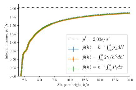
**Figure 6.** Integral pressure  $\hat{p}$  as a function of slit pore height h. The integral pressure is computed as the average tangential mechanical pressure, see Equation (34), and from the normal pressure and surface tension, see Equation (39).
