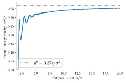
**Figure 5.** Internal energy density u = U/V as a function of slit pore height h. See Equation (35). The dashed line shows the internal energy density of the bulk  $u^b$ .
