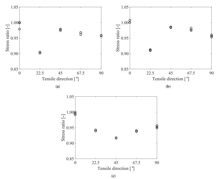
**Figure 9.** Stress ratio versus tensile direction from the tensile tests on the smooth specimen in the various tensile directions of alloy (**a**) AA6061, (**b**) AA6063 and (**c**) AA6110.
