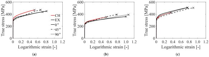
**Figure 16.** Representative stress-strain curves from the tension tests on the smooth specimen for the three alloys in the extruded (EX) and the cast and homogenized (CH) conditions. The stress-strain curves of the two conditions are compared for each alloy: (a) AA6061, (b) AA6063 and (c) AA6110. The legend in sub-figure (a) is valid for all sub-figures.
