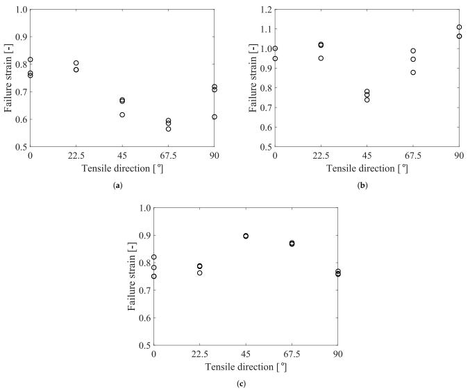
**Figure 11.** Failure strain versus tensile direction from the tensile tests on the smooth specimen of the alloys (**a**) AA6061, (**b**) AA6063 and (**c**) AA6110.
