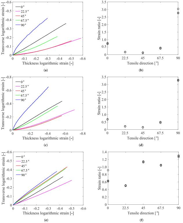
**Figure 10.** Transverse versus thickness strain curves plotted to failure (left column) for the alloys (**a**) AA6061, (**c**) AA6063 and (**e**) AA6110, and average strain ratio (*R*-value) up to necking versus tensile direction (right column) for the alloys (**b**) AA6061, (**d**) AA6063 and (**f**) AA6110, all taken from the tensile tests on the smooth specimen for the three alloys.
