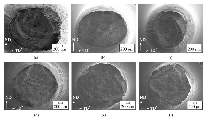
**Figure 12.** Fracture surfaces of representative tension tests for alloy AA6061. (a) Smooth,  $0^{\circ}$ , (b) Smooth,  $45^{\circ}$ , (c) Smooth,  $90^{\circ}$ , (d) R0.8,  $0^{\circ}$ , (e) R0.8,  $45^{\circ}$ , (f) R0.8,  $90^{\circ}$ .
