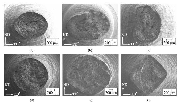
**Figure 13.** Fracture surfaces of representative tension tests for alloy AA6063. (a) Smooth, 0°, (b) Smooth, 45°, (c) Smooth, 90°, (d) R0.8, 0°, (e) R0.8, 45°, (f) R0.8, 90°.
