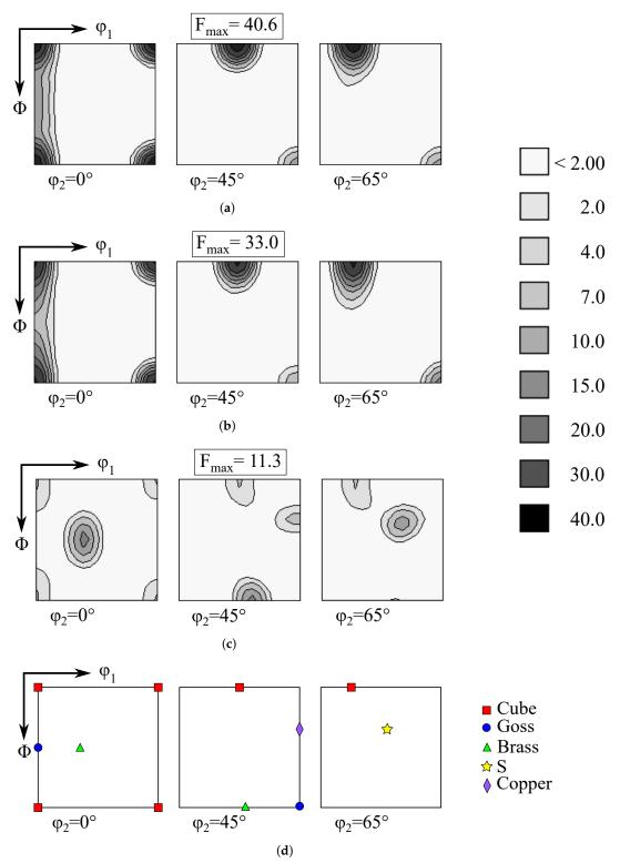
**Figure 6.** Orientation distribution functions (ODFs) for the alloys (**a**) AA6061, (**b**) AA6063 and (**c**) AA6110, indicating their crystallographic texture, where (**d**) show the location of the individual texture components. The scale bar gives the intensity of the function, where the maximum intensity  $F_{max}$  of the ODF is given at the top of each sub-figure.
