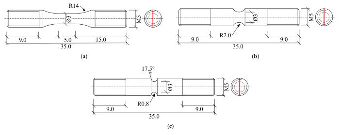
**Figure 2.** Nominal geometries of the (**a**) smooth, (**b**) notch R2.0 and (**c**) notch R0.8 tension test specimens. The red line in the rightmost figure in each sub-figure represents the ND of the extruded profile, and was marked physically on the specimens. All measures are in mm.
