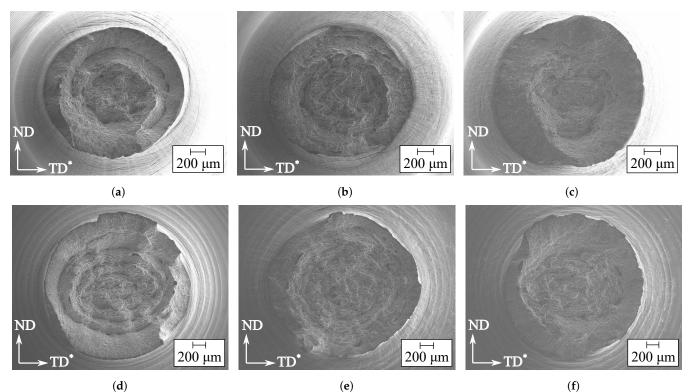
**Figure 14.** Fracture surfaces of representative tension tests for alloy AA6110. (a) Smooth,  $0^{\circ}$ , (b) Smooth,  $45^{\circ}$ , (c) Smooth,  $90^{\circ}$ , (d) R0.8,  $0^{\circ}$ , (e) R0.8,  $45^{\circ}$ , (f) R0.8,  $90^{\circ}$ .
