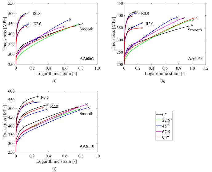
**Figure 7.** Representative stress-strain curves for all tested combinations of tensile direction and specimen geometry of alloy (a) AA6061, (b) AA6063 and (c) AA6110. The  $\times$  marks failure at maximum true stress.
