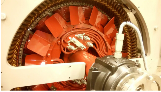
Fig. 3. The experimental set-up of 100 kVA custom-made synchronous generator for the purpose of fault detection (top), the rotor of the generator and the taps of field winding to apply ITSC fault.
