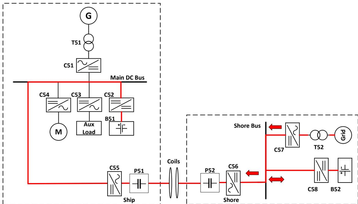
Figure 3: Inductive shore-to-ship charging for a DC-microgrid-based propulsion system
