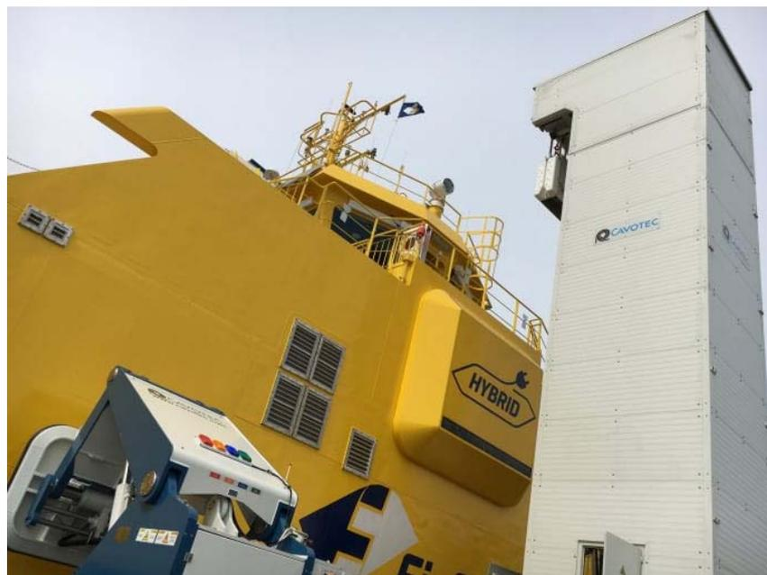
Figure 8: Cavotec APS tower used for charging MF Elektra. Photo: Cavotec
