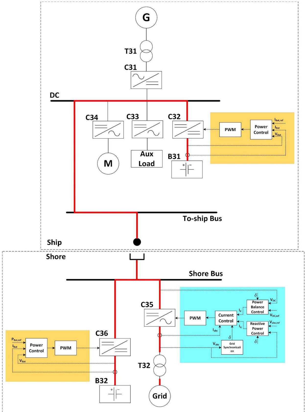
Figure 15. Converter control for charging path
