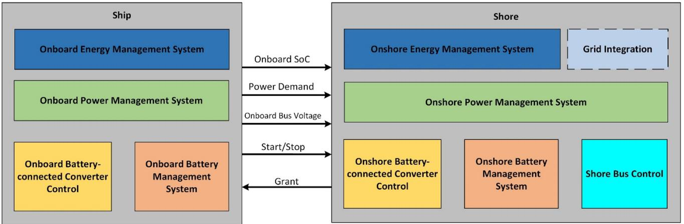
Figure 16. An example of the system-level control structure
