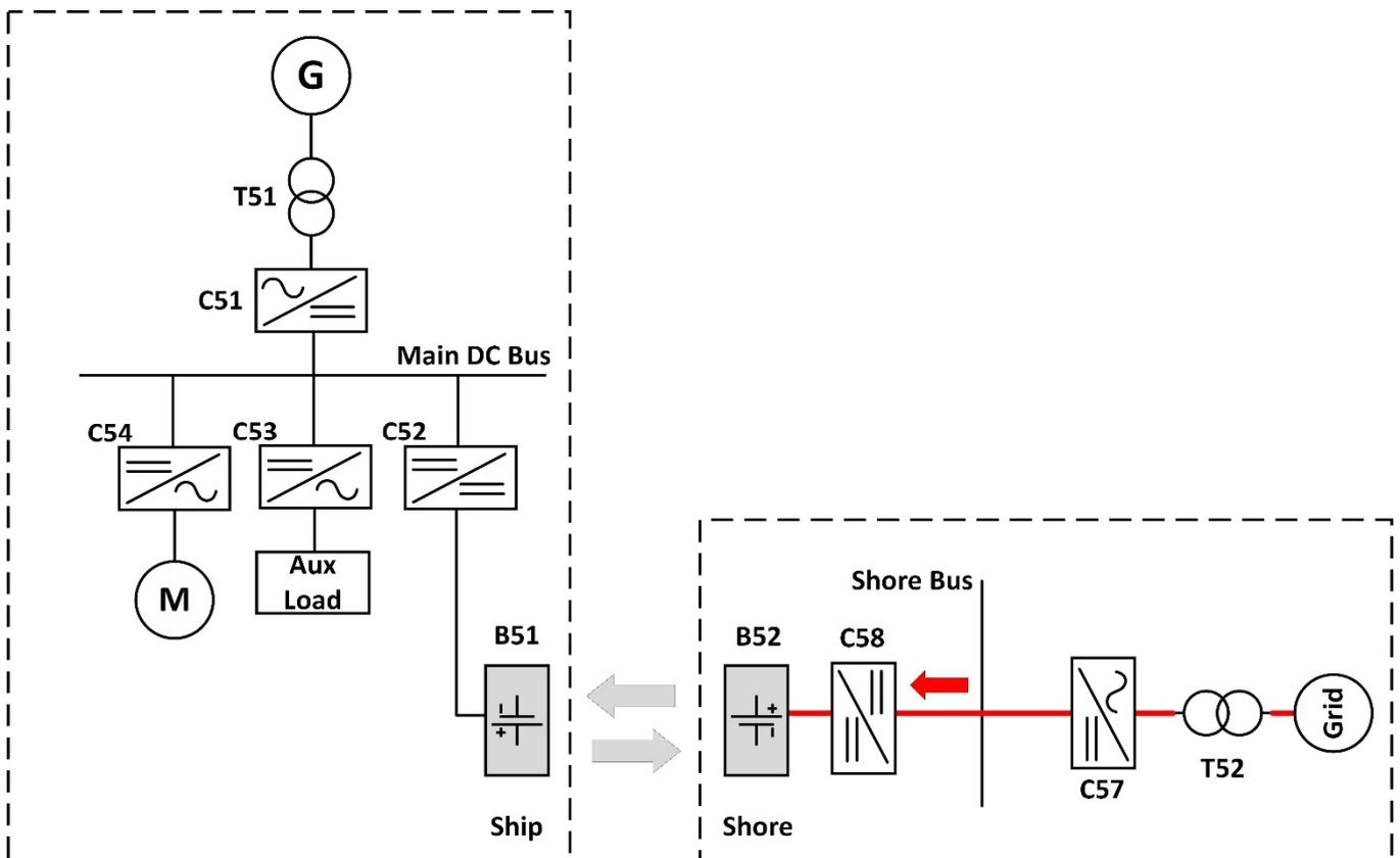
Figure 4: Battery swapping method
