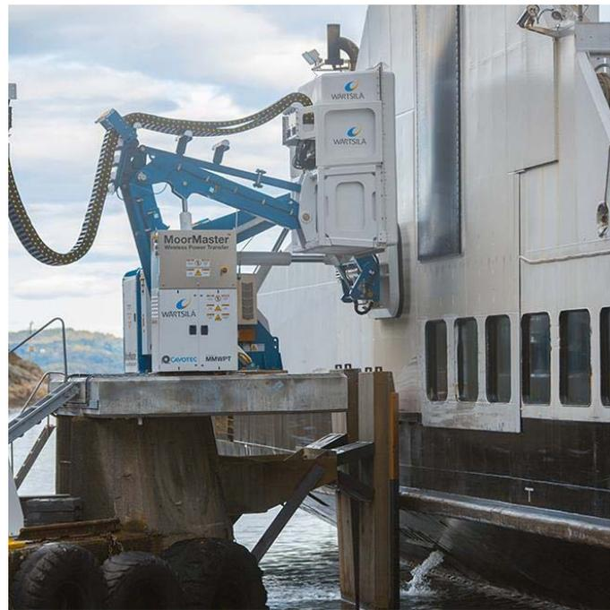
Figure 13: Wartsila Inductive charging system for charging MF Folgefonn. Photo: Wartsila
