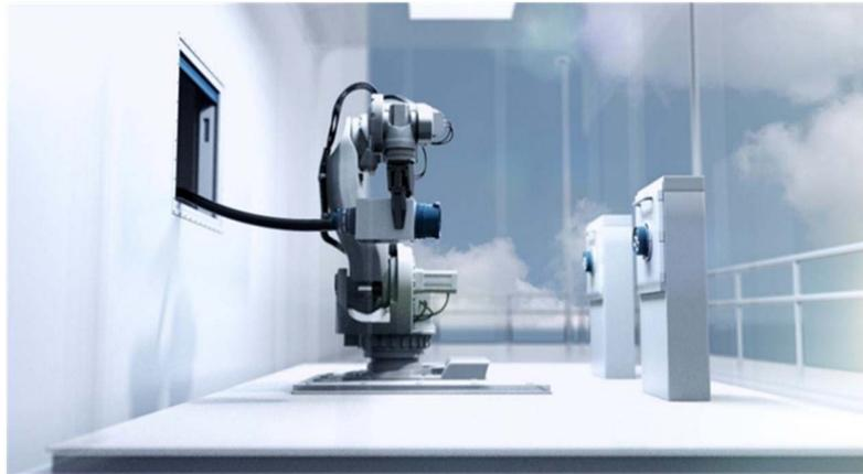
Figure 7: ABB IRB7600, an autonomous robotic arm used for charging MF Aurora and MF Tycho Brahe. Photo: ABB
