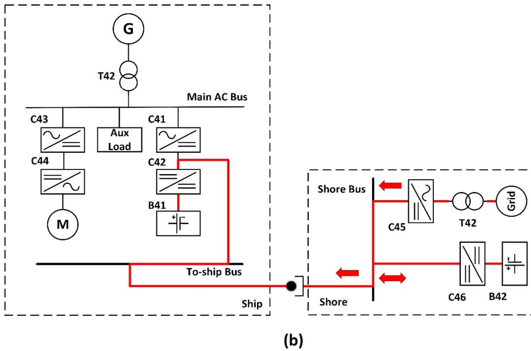
Figure 2: DC shore-to-ship charging for (a) a DC-microgrid-based and (b) an AC-microgrid-based propulsion system
