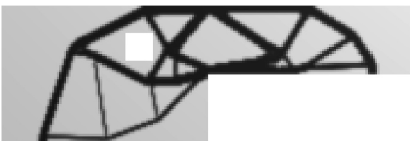
Fig. 3. Optimized topology of the dapped-end beam. Black and grey pixels indicate the solid and void regions.
