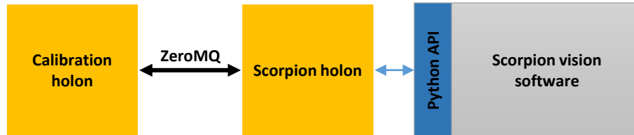
Figure 26: Architecture of a holonic-based calibration service
