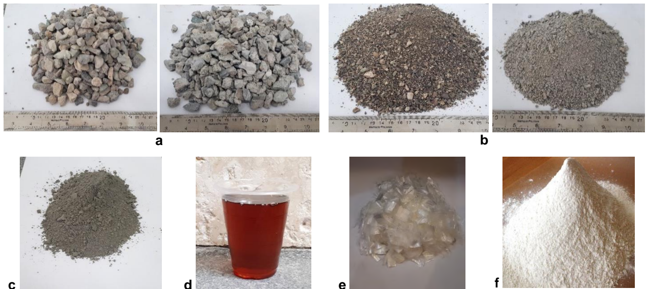
Figure 2. Materials; a) natural and recycle coarse aggregate; b) natural and recycle fine aggregate; c) cement; d) superplasticizer (SP); e) fiber; f) limestone.
