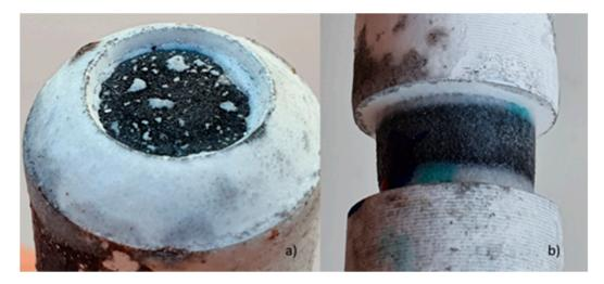
Figure 13. Images of anodes after experiment: (a) horizontal anode and (b) vertical anode.
