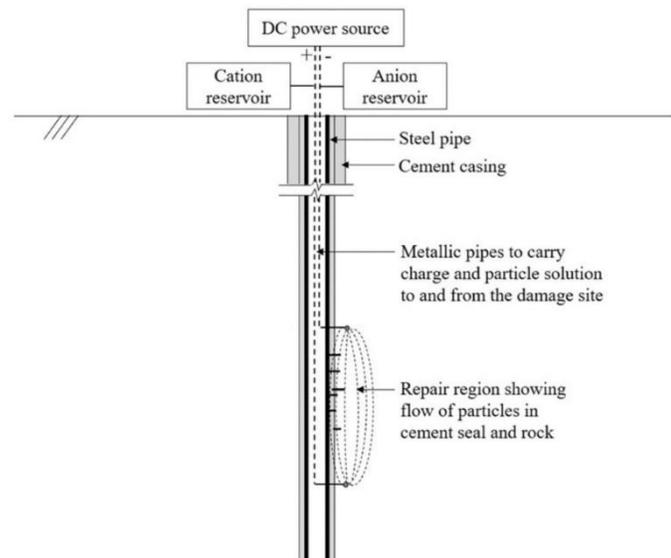
Figure 9: Proposed method applied to a wellbore [85].
