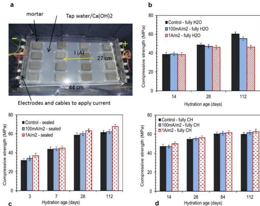
**Figure 4:** a) Experimental set-up for DC curing of samples submerged in water and  $\text{Ca}(\text{OH})_2$  solution [50]. Compressive strength as a function of curing time for mortar samples under current flow conditions: b) submerged in  $\text{H}_2\text{O}$ ; c) sealed condition; d) submerged in  $\text{Ca}(\text{OH})_2$  solution [49].
