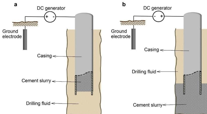
Fig. 8: Schematic view of the well showing the apparatus for: a) cleaning the casing from the drilling mud; b) increasing the bonding of cement to casing by DC field application, after [80].
