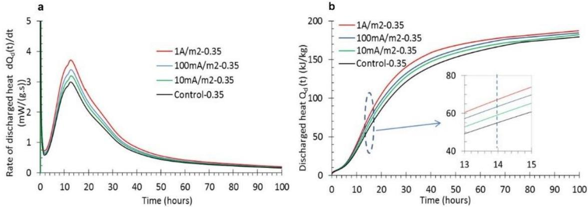
**Figure 3:** Impact of current flow level on hydration of cement paste with w/c ratio of 0.35 measured by isothermal calorimetry at 20 °C; a) rate of discharged heat, and b) cumulative amount of discharged heat [47].
