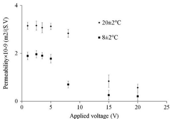
**Figure 6:** Electroosmotic permeability as a function of applied voltage [39].
