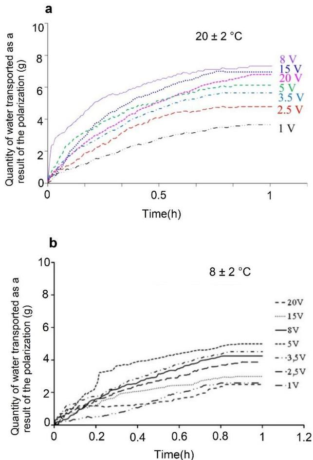
**Figure 5:** The quantity of transported water over time as a function of applied voltage at ambient temperature of: a)  $20 \pm 2$  °C [40], and b)  $8 \pm 2$  °C [39].
