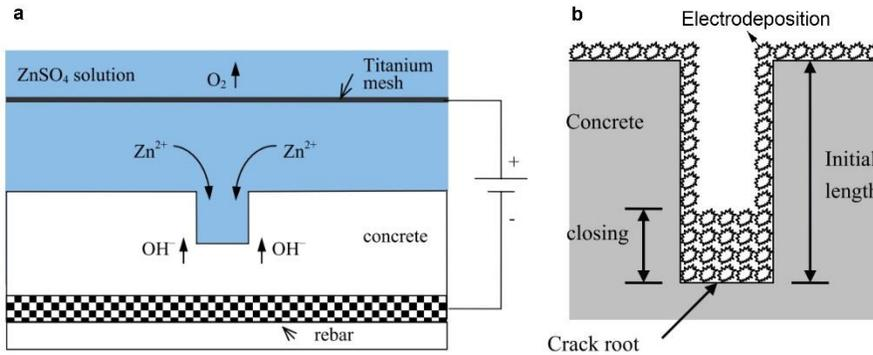
**Figure 7:** Suggested mechanism of electrodeposition of ZnO from ZnSO<sub>4</sub> solution. Schematic illustration of: a) the set-up ; and b) the deposition mechanism, which starts from the root of the crack and piles up to the surface. [67]
