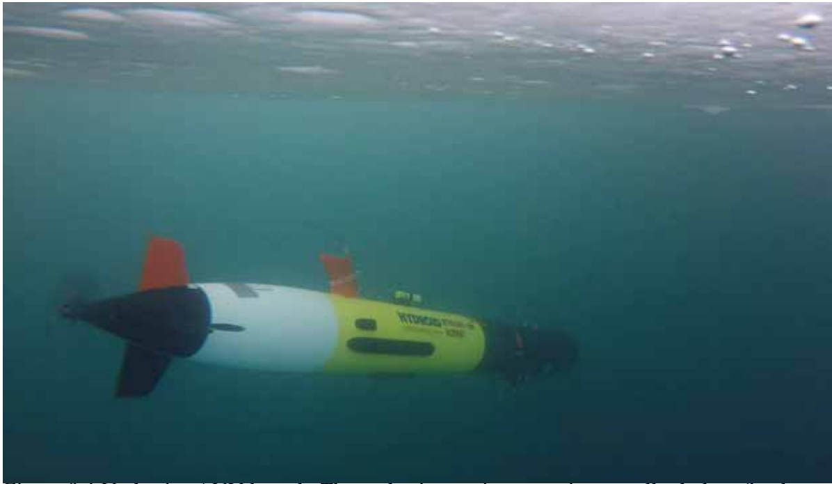
Figure 9.6 Under-ice AUV launch. The under-ice environment is normally dark as for the polar night operations in open waters.
