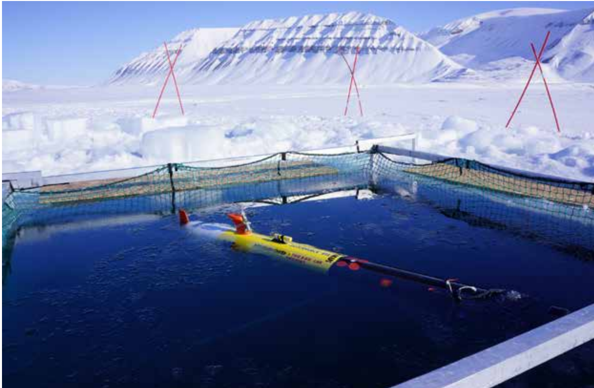
Figure 9.5 The REMUS 100 ready for under-ice missions.
