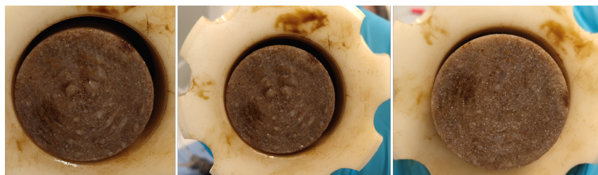
Figure 6. Physical filtration and formation of nanoparticle “cake” at core inlet during nanofluid flooding.
