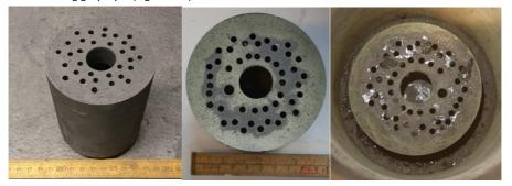
Figure 227: Left: Gas production chamber before Exp. 3a; Center: Top view of green layer on gas production chamber, Exp. 1a; Right: Top view of green and grey layer on gas production chamber, Exp. IF2a.
