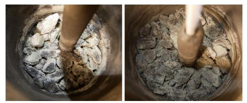
Figure 167: Left: Stoking point Y = 21 cm, T=1420°C, Exp IF75-7a. Right: Brown condensates at Y = 18 cm, T = 1580°C for experiment IF75-7a.
