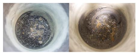
Figure 177: Brown partially reacted pellets leftovers, Exp. IF5a (left) and IF6a (right).
