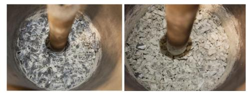
Figure 166: Excavation of the crucible at Y = 18 cm, T = 1485°C. SiC charge before (left) and after poking (right), experiment IF2a.
