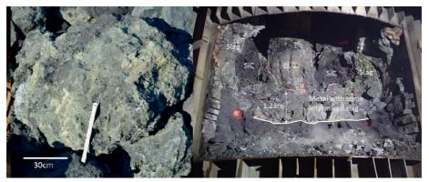
Figure 37: Side crust [2]; Material zones observed in the furnace during excavation. Electrode 1 is visible in the middle of the picture, and SiC, slag and metal zones are indicated [60].
