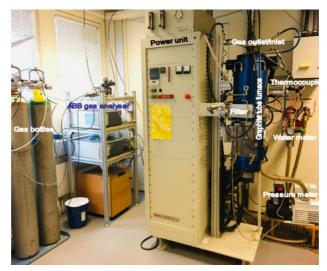
Figure 82: Graphite tube furnace (Thermal Technology model 1000-3560-FP20) [22].
