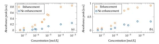
**Figure 9.** The absorption peak values for (**a**) R6G and (**b**) CV measured with the tapered fiber with and without a 100 nm Au film. The absorption signal was stabilized before it was collected.
