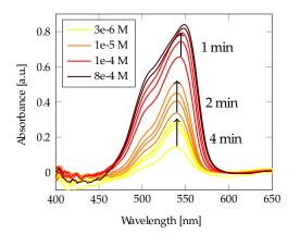
**Figure 6.** R6G measured with time from a 100 nm Au film on the taper. For each measurement, the signal increased with time until it stabilized.
