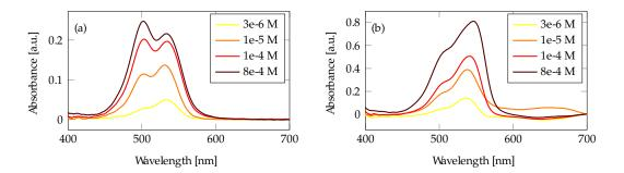
**Figure 5.** R6G measurements in a tapered fiber: (**a**) without Au film and enhancement, and (**b**) with Au film and enhancement.
