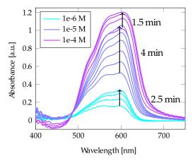
**Figure 8.** A 100 nm Au film on the taper displayed enhancement of the absorption signal of CV. The signal increased until saturation.
