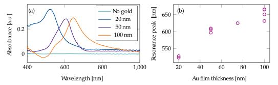
**Figure 4.** (a) examples of the characterization of a resonance wavelength measured in water with air as reference for 20 nm, 50 nm, and 100 nm Au films. The spectrum from a tapered fiber without an Au film is plotted for comparison; (b) resonance wavelength as a function of Au thickness.
