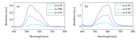
**Figure 7.** Crystal Violet (CV) measurements in a tapered fiber: (**a**) without Au film and (**b**) with a 100 nm Au film and enhancement.
