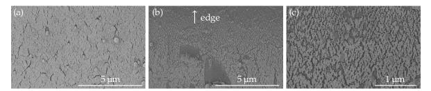
**Figure 2.** SEM images of the deposited 100 nm Au film. (**a**) the center of the film is almost continuous; (**b**) the film thins towards the edge of the deposition layer; (**c**) a closer look at the thinner part of the film towards the edge.
