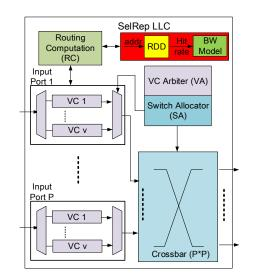
Fig. 8: A block diagram of an MC-router that supports SelRep LLC. SelRep LLC minorly modifies the router by adding the RDD and bandwidth model logic (both structures are off the critical path).
