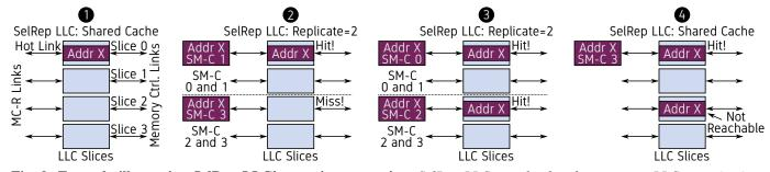
Fig. 9: Example illustrating SelRep LLC's run-time operation. SelRep LLC seamlessly adapts to new LLC organizations by lazily and selectively replicating cache blocks.
