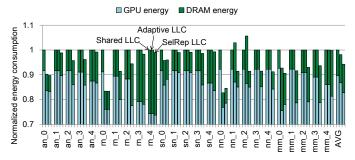
**Fig. 16: Normalized energy consumption.** SelRep LLC reduces energy consumption by 5.7% on average compared relative to the shared cache configuration.
