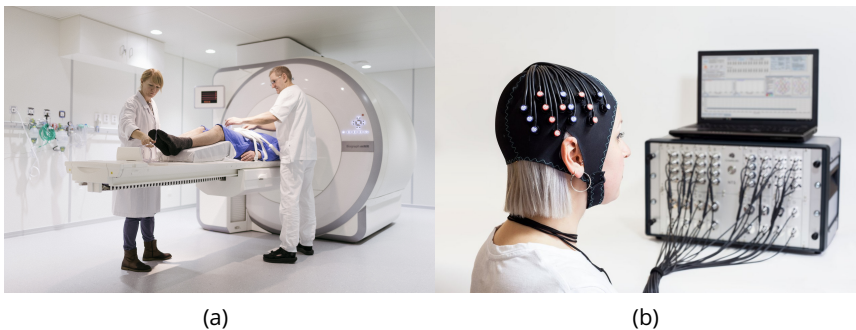
Figure 2.2: Methods for measuring brain activity using blood flow (a) functional magnetic resonance imaging and (b) functional near-infrared spectroscopy.
