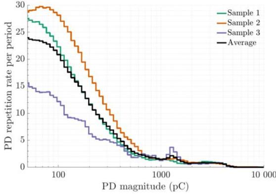
b) Bars close to the high voltage terminal. The void gap distance  $d_c$  was adjusted to 0.3 mm to correlate model and experimental results.
