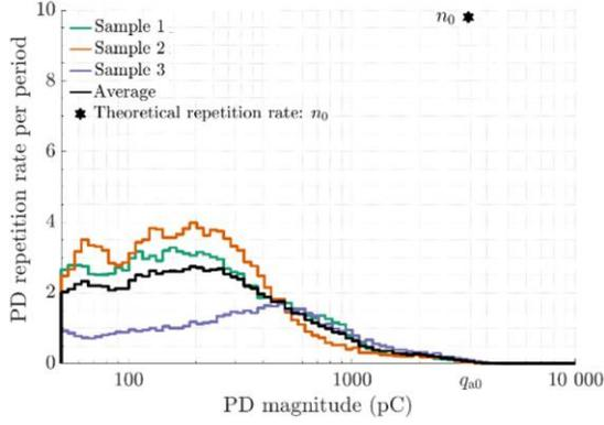
a) Laboratory object with void diameter of 10 mm and void gap distance of 0.5 mm. The expected PD repetition rate is indicated by a star.
