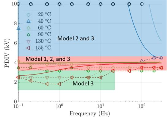
a) Laboratory object with void diameter of 10 mm and void gap distance of 0.5 mm. Black markers at 10 kV indicates no PDIV measured.
