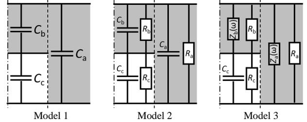
Fig. 1. Three electrical models used for pd-modelling of test object, a) represents the classical capacitive abc-model b) resistance and c) the impedance model.
