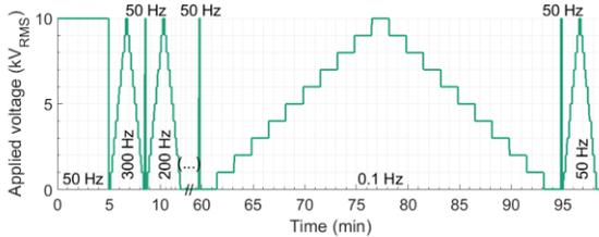
Fig. 4. Sketch of the voltage application frequency sweep with reducing frequency. This sketched procedure was used on the laboratory objects, whereas the start frequency for the bars was 50 Hz due to a higher capacitance and limited available current in the voltage source.
