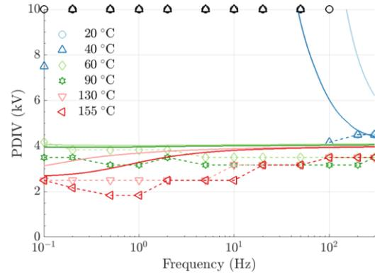
a) Laboratory object with void diameter of 10 mm and void gap distance of 0.5 mm. Black markers at 10 kV indicates no PDIV measured.
