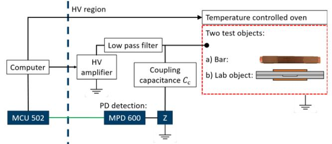
Fig. 3. Test setup for PD measurements
