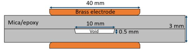
a) Laboratory made [Not to scale] 3 mm thick object with a void with diameter of 10 mm and a gap distance of 0.5 mm.
