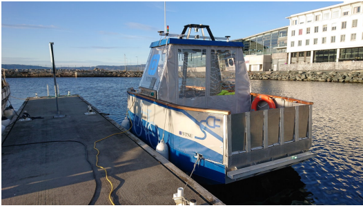
Fig. 1: The experimental autonomous urban passenger ferry milliAmpere .
