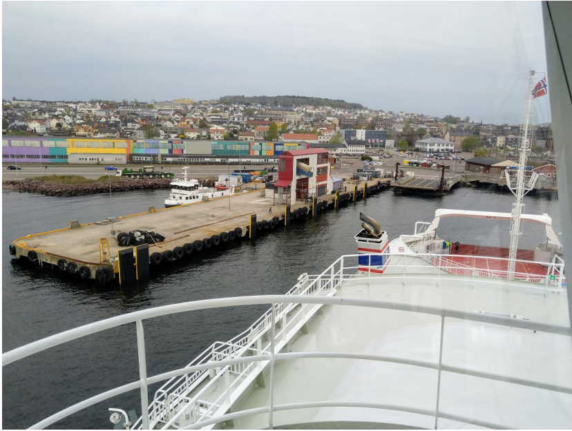
Figure 2.10: Bastø VI docking automatically in Horten, Norway in 2019 by using technology from Kongsberg Maritime.
