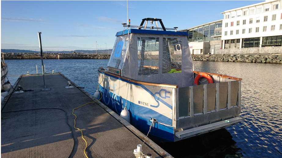
Figure 2.1: The experimental electric autonomous passenger ferry milliAmpere .
