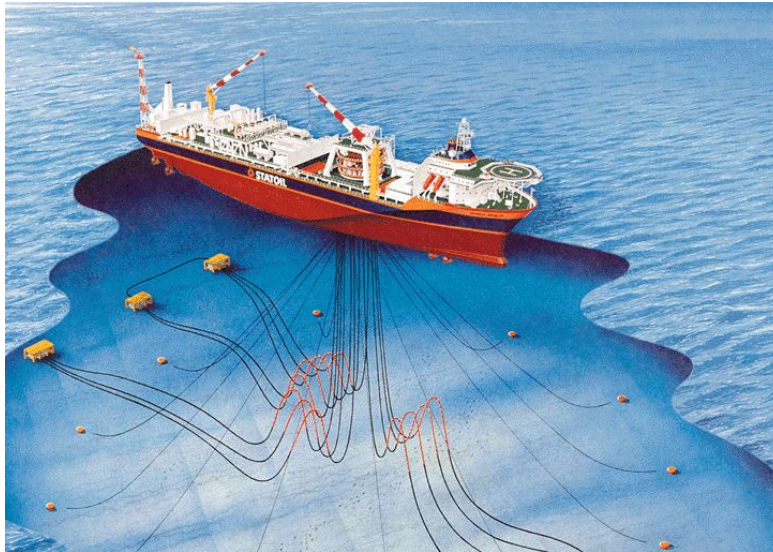
Figure 3: Illustration of the Norne 6608/10 FPSO (Courtesy: Equinor).
