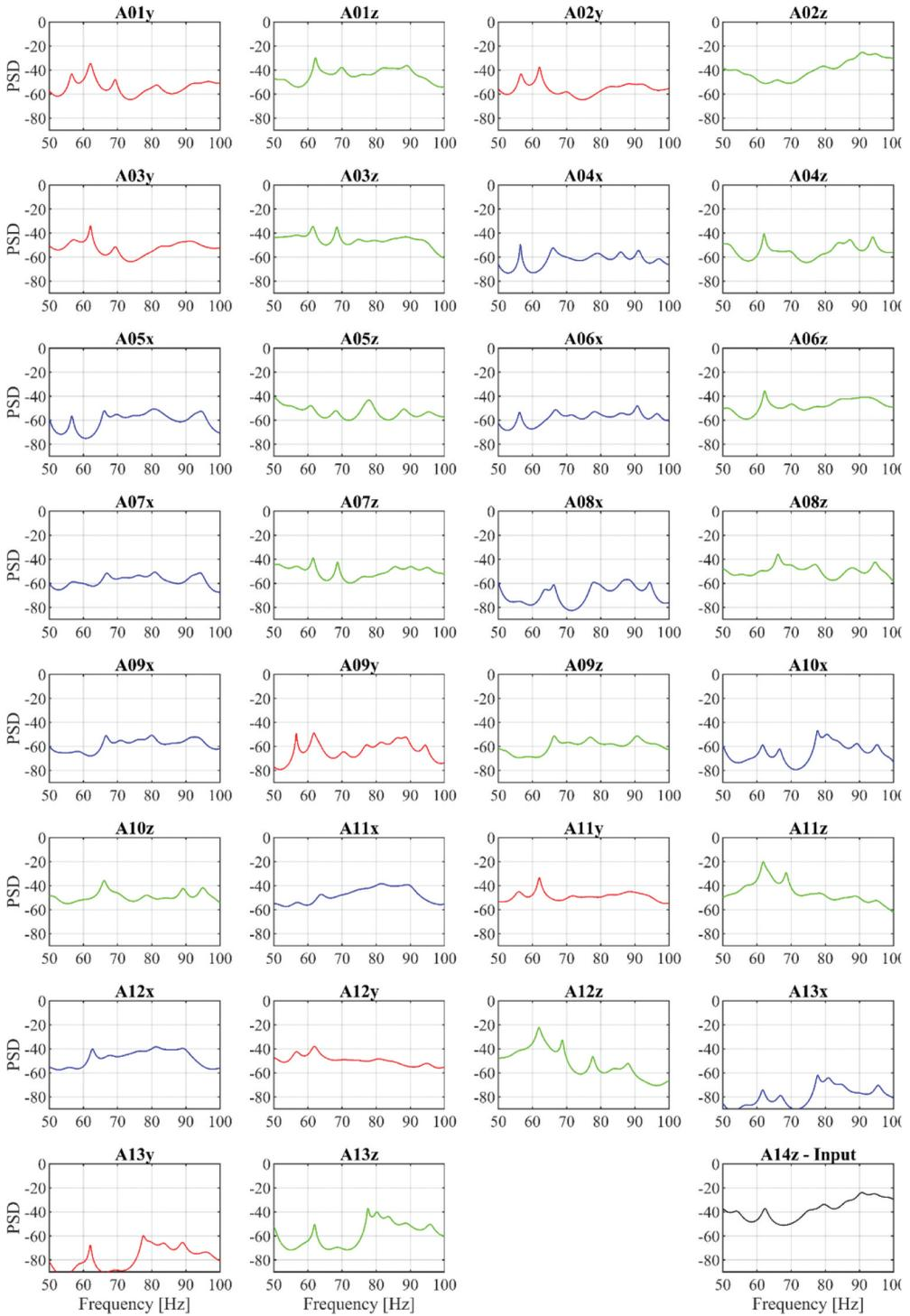
**Figure 5.** Logarithmic PSD of acceleration time series from four sine sweeps, 50–100 Hz.
