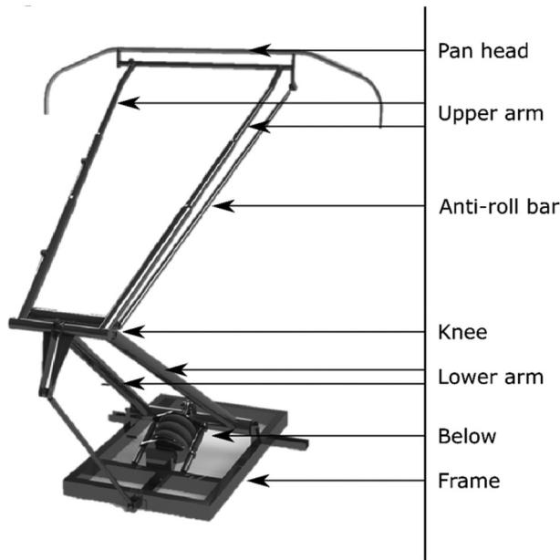
**Figure 7.** Overview of pantograph parts and the naming used in the component study.
