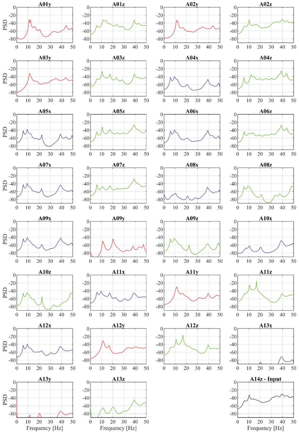
**Figure 3.** Logarithmic PSD of acceleration time series from four sine sweeps, 0–50 Hz.
