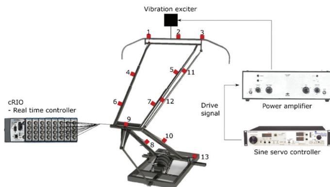
**Figure 2.** Laboratory pantograph experimental setup and position of accelerometers. Sensor 14 was mounted on the actuator.
