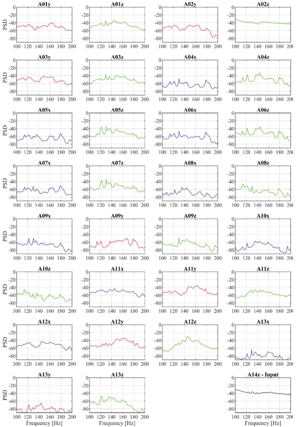
**Figure 6.** Logarithmic PSD of acceleration time series from four sine sweeps, 100–200 Hz.
