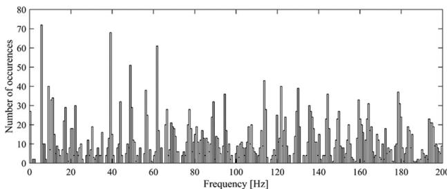
**Figure 4.** Histogram of all the peaks from the logarithmic PSD of all time series; 4 tests, 32 channels, approx. 3200 peaks from 0 to 200 Hz.
