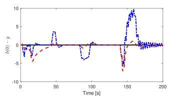
Fig. 2: Case 1: Tracking error for the old (blue) and new (red) methods.
