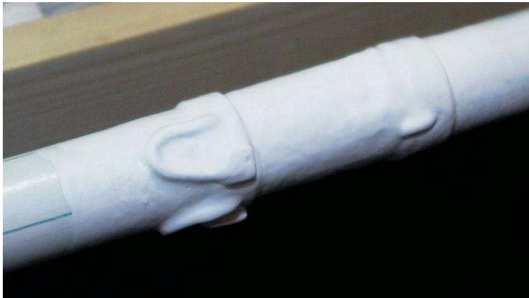
Figure 3.4: Riser instrumentation, strain gauge to the right and accelerometer to the left (Braaten and Lie, 2005).
