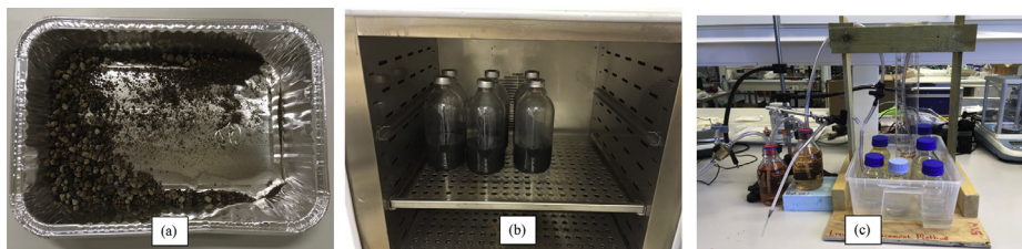
Fig. 1. Snapshots of some experimental steps: (a) oven-dried olive cake; (b) incubator with a few reactor bottles; and (c) water displacement apparatus for volumetric biogas measurement.
