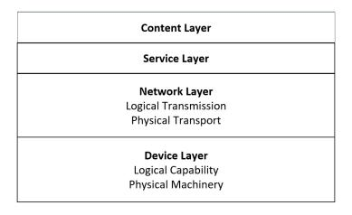
Figure 3. The layer architecture of digital technology adopted from (Yoo et al., 2010)
