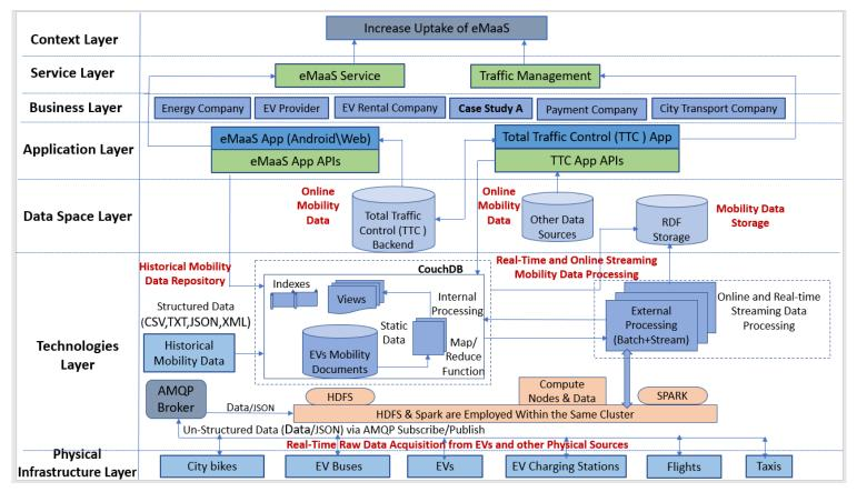
Figure 9. Mobility data (history, real-time, and online) processing in the architecture
