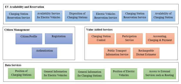
Figure 2. Overview of eMaaS adapted from (Tcholtchev et al., 2014)
