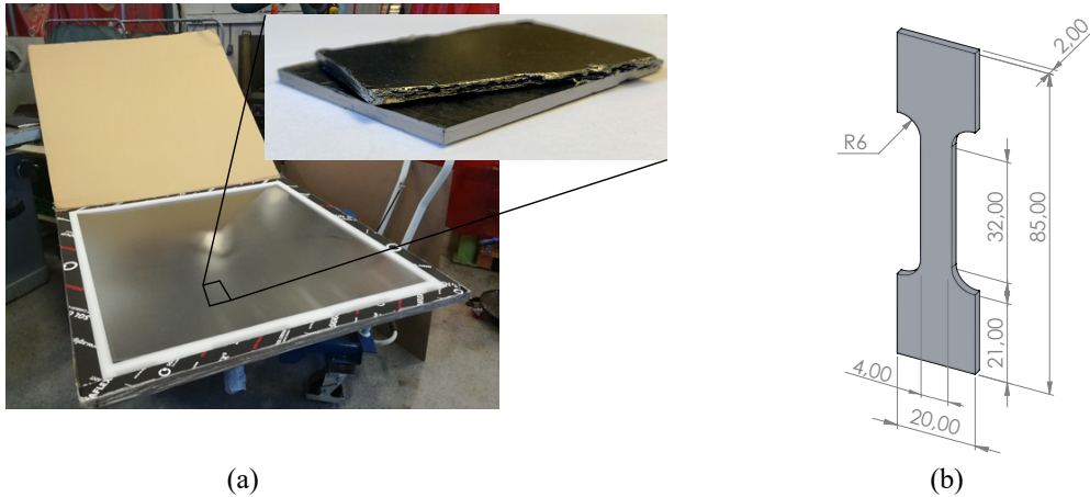
Fig. 2: (a) Sigraflex® foils as delivered with magnification view and (b) specimen geometry and dimensions [mm].
