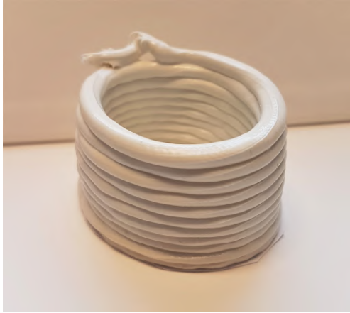
Fig. 1. Proof-of-concept: Structure built with helix-path, but with a strictly vertical orientation of the tool (Evjemo et al., 2017).
