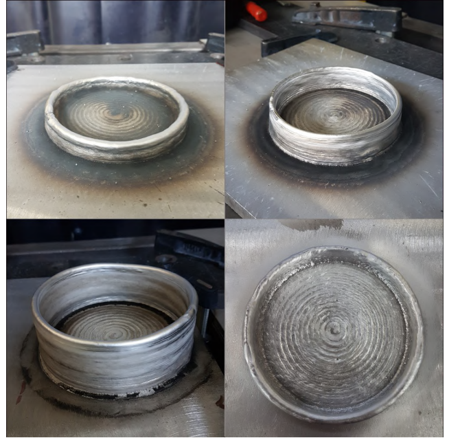
Fig. 5. Set-based control: The structures built in the first three tests, and close-up of the bottom.
