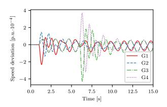
Fig. 1. The speed response obtained from the linear simulation of a model of the Kundur Two-Area System is shown.
