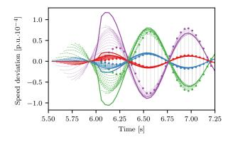
Fig. 2. The oscillations caused by the second local mode, involving  $G_3$  &  $G_4$ , are shown (where the same colors as those in Fig. 1 are used for each generator). The four thick lines shows the oscillations for each generator computed using the linear model. The thin lines show the fitted curves for each time instant, and the markers correspond to the instantaneous estimate at that time.
