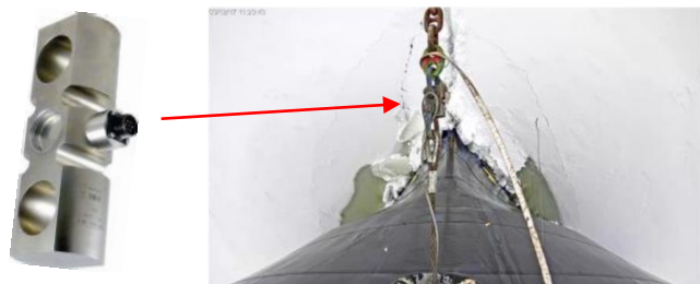
(a) Location of load cell in the mooring line [15]
