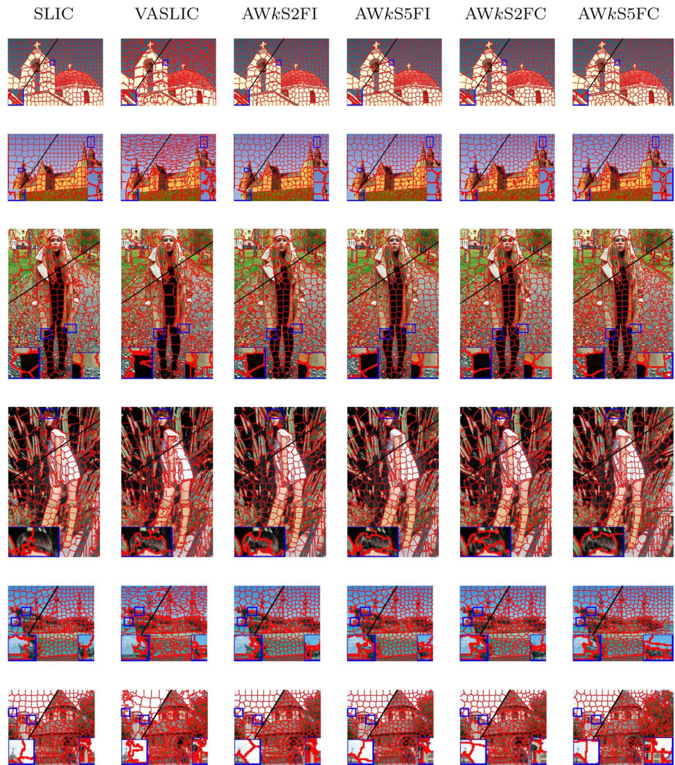
Fig. 3 Visual comparison among SLIC [1], VASLIC [25] and four configurations of AWkS algorithms. Test images belong to [row 1 and row 2] BSDS500 Dataset [34], [row 3 and row 4] FASH Dataset [36], and [row 5 and row 6] SBD Dataset [35]. Fragments forming the images above have k \approx 250 in the upperleft corner and k \approx 500 in the lower right corner
