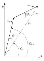
Fig. 2: The heading angles  $\psi^\pm_{\rm ca}$  can be found geometrically by the computation of  $\phi^\pm.$
