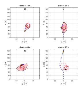
Fig. 3: The first scenario. The vehicle is the orange polygon and the obstacle is the red circle. The magenta circle represents the radius  $R_{\rm o|\epsilon}$ . The obstacle and vehicle trajectories are the red and blue dashed lines, respectively. The target position,  $p_{\rm t}$ , is marked as an 'X'. The blue arrow represents  $v_{\rm dgr}$ , and the red cone represents  $\mathcal{CC}_{\rm o|\epsilon}$  with length  $d_{\rm threshold}$ .
