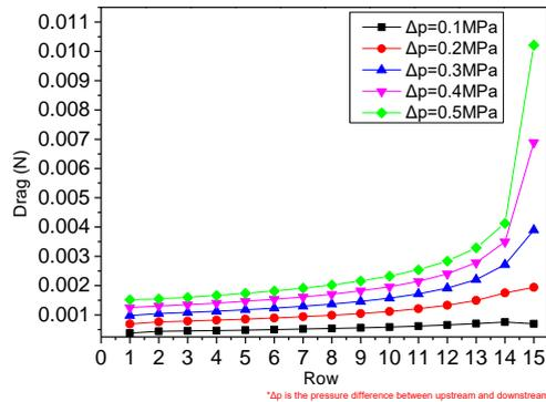
**Fig.4.** The change curve of drag of bristles ( $S_D/d=1.10$ )
