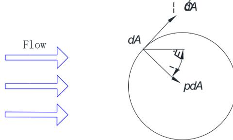
**Fig. 3.** The pressure drag acting on the body
