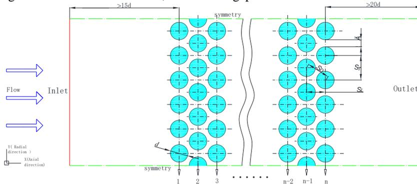
**Fig. 1.** The sketch of 2-D staggered arrangement of tube bank model
