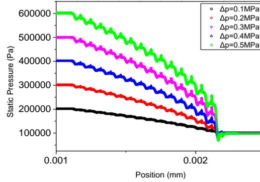
**Fig. 5.** Pressure distribution along axial gap of bristle under pressure differentials
