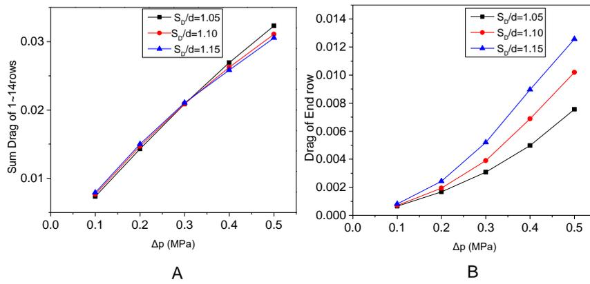
**Fig. 6.** The drags in the front rows (A) and the end row (B)
