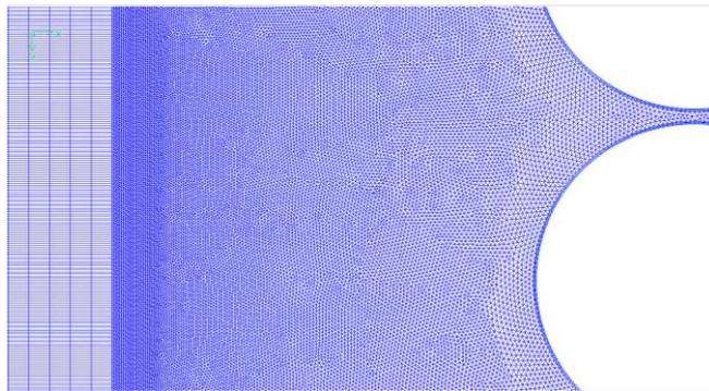
**Fig. 2.** The structure of mesh
