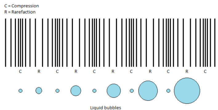
Figure 1. Ultrasonic pressure wave propagation and growth of a cavitation bubble during some cycles of ultrasound [13].
