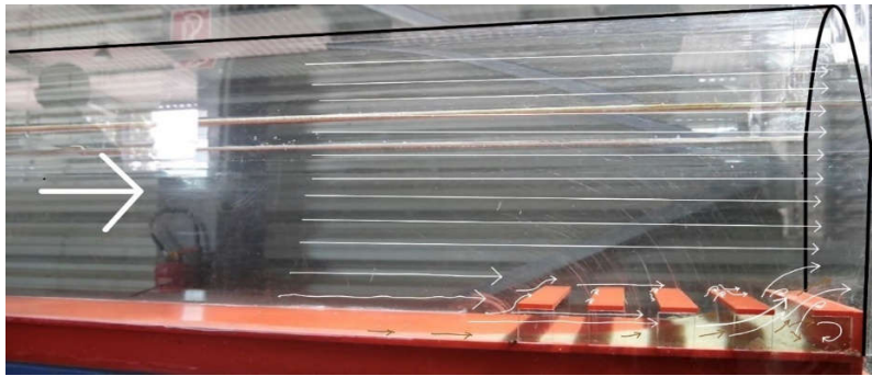
Figure 22: Snapshot of the sand transport from a test with ribs without a ramp (0% trap efficiency)
