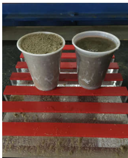
Figure 24: Comparison of the injected and trapped sand from a test with ribs and a ramp
