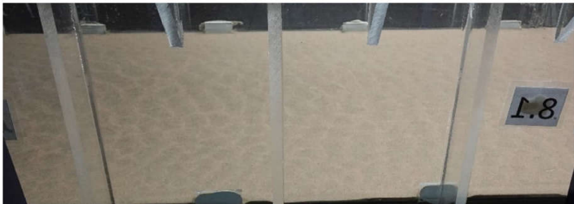
Figure 17: Sand deposition after the test of the existing situation
