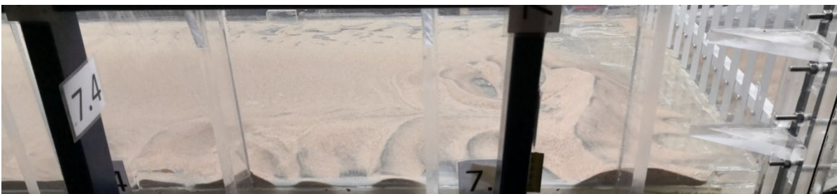
Figure 43: Deposition pattern at the start of the sand trap after modification 1
