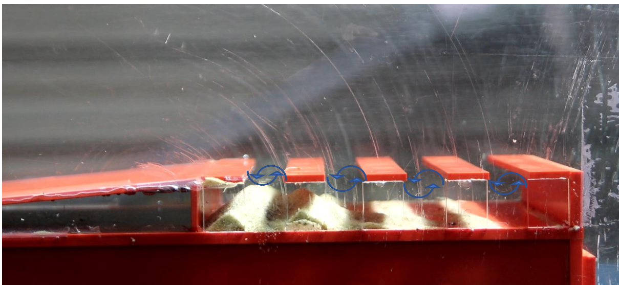
Figure 264: Result with 60 l/s resp. 80 m 3 /s for prototype with sand 0.3-1.0 mm
