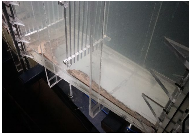
Figure 57: Sediment deposits seen in the sand trap transition
