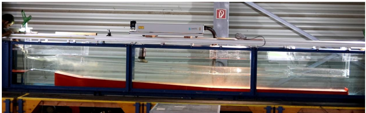
Figure 232: Discharge 41 L/s, sand inflow 0.5 L, sand from above, snapshot 21 s
