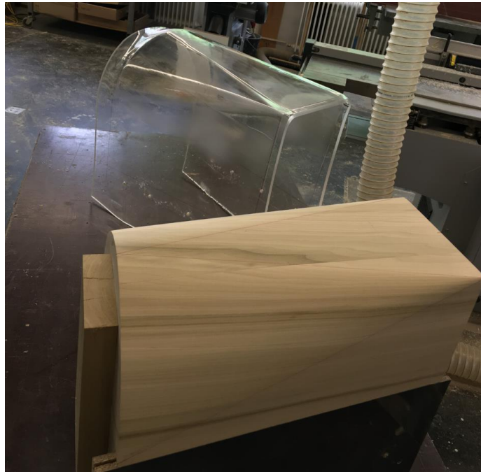
Figure 210: 3D geometry realization in plexiglass 1:36.67
