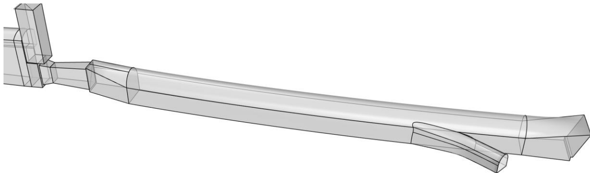
Figure 8: Sand trap geometry from design plans
