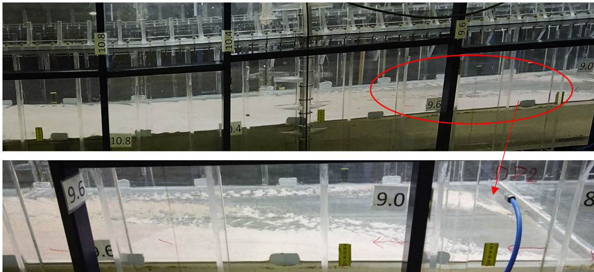
Figure 29: Erosion/deposition pattern after sand trap filling test
