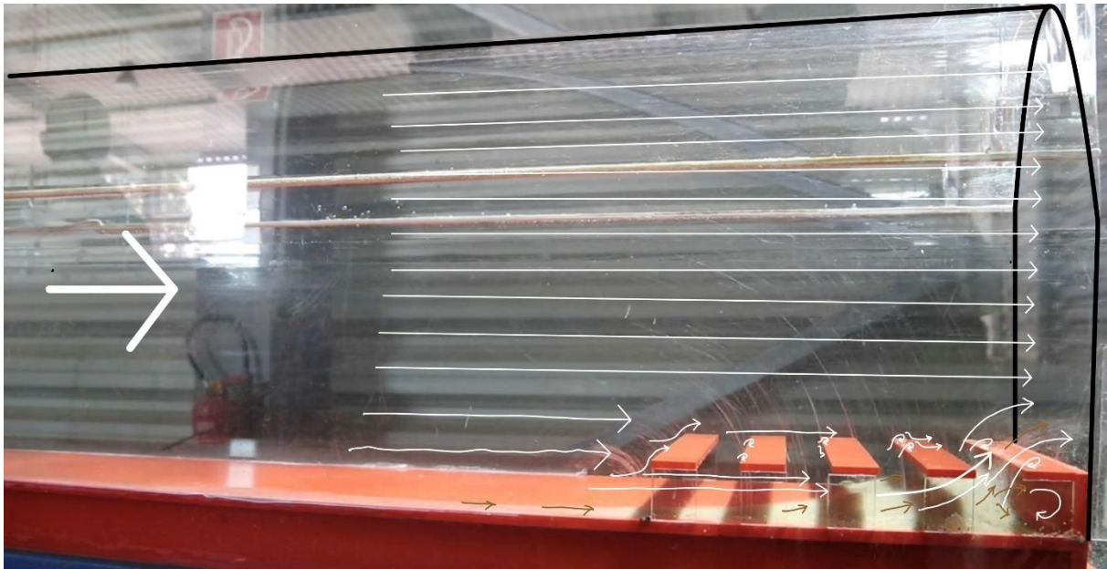
Figure 259: Flow visualization with sand transport under the ribs
