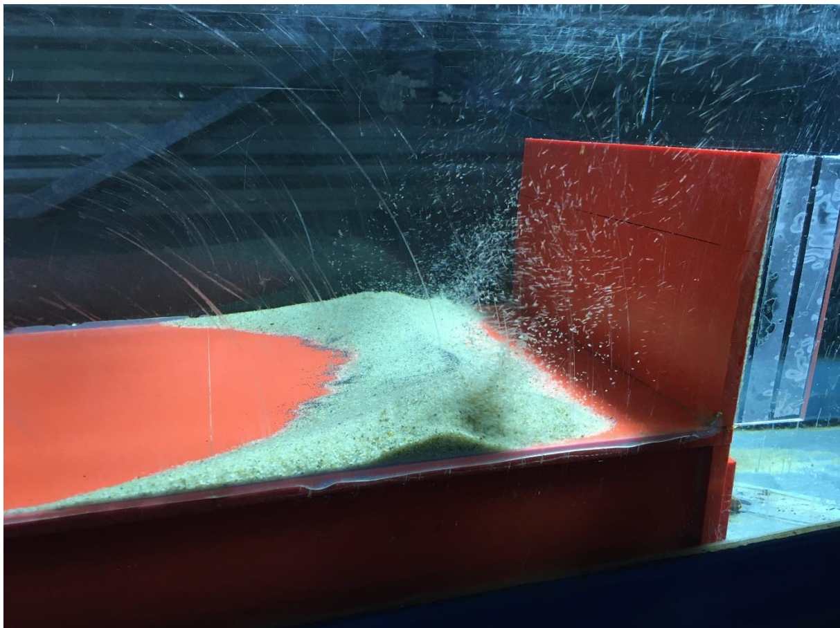
Figure 241: Discharge 48 L/s, weir height 3.0 [-], sand inflow 0.5 L, sand overtopping weir downstream, snapshot
