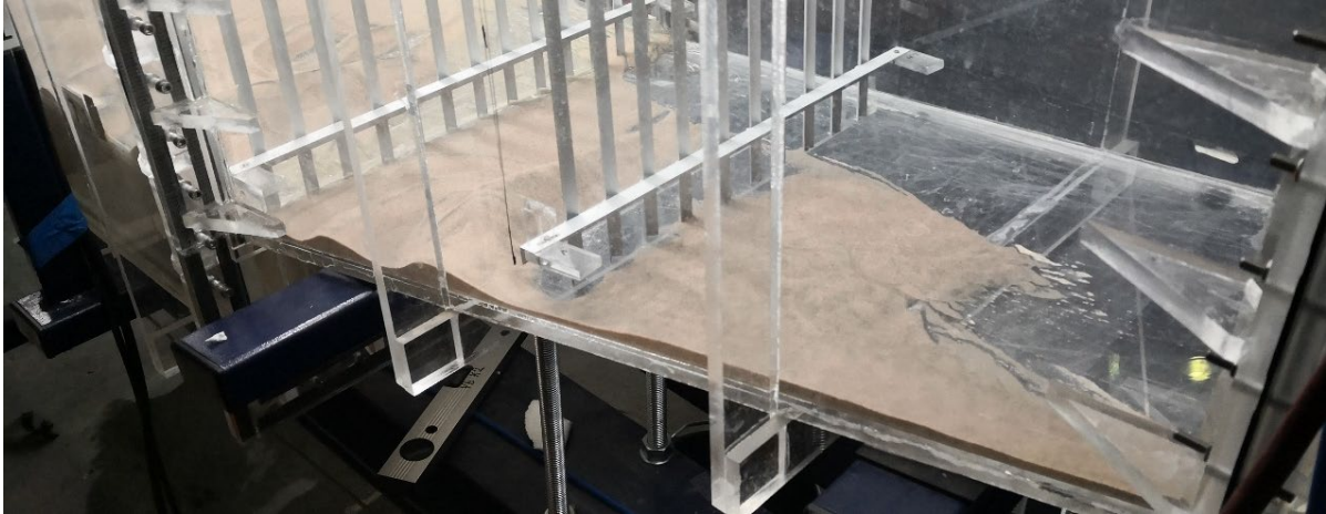
Figure 42: Deposition pattern at the sand trap transition after modification 1
