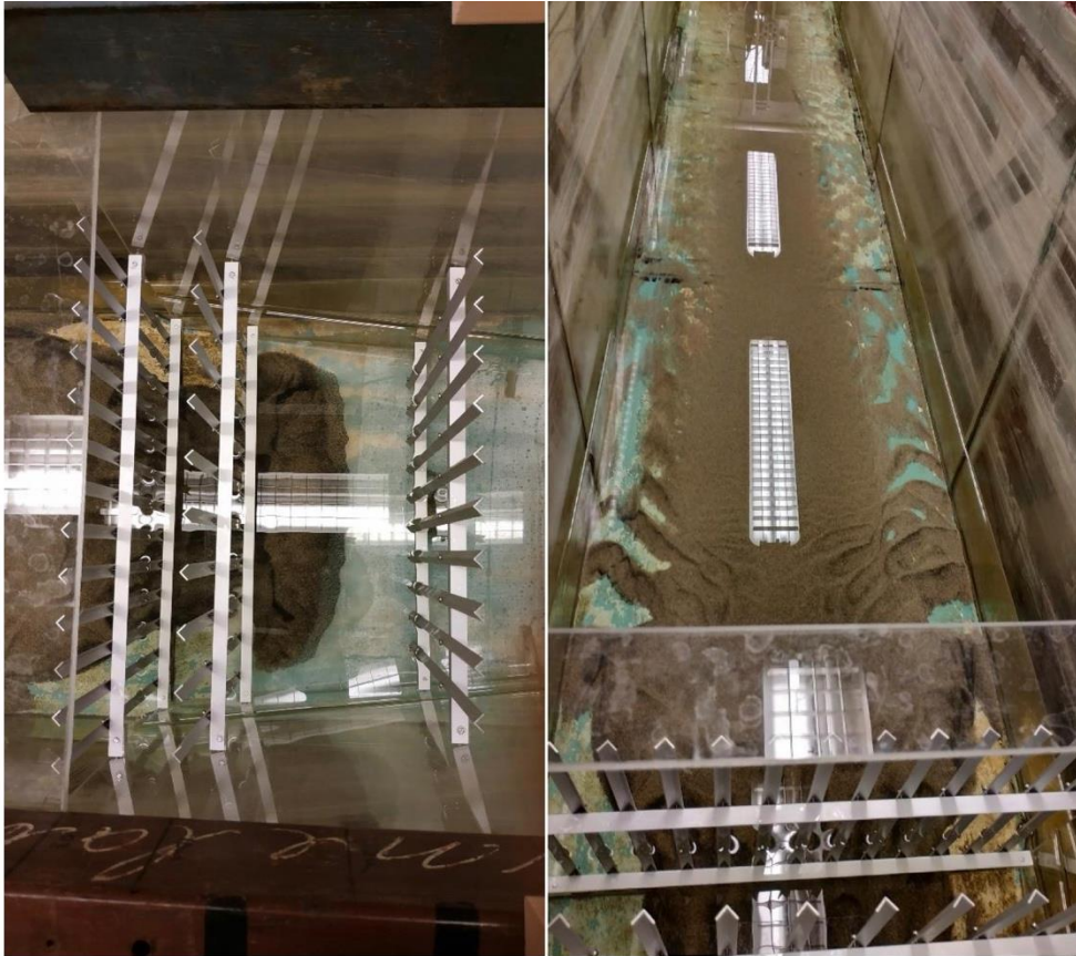
Figure 3: Flow calming device studied by Daxnerová at NTNU (Daxnerová 2019)
