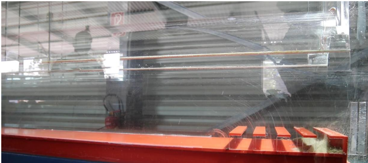
Figure 256: 59.6 l/s, sand transport moving the dune under rib No.1 – constant flushing of sand directly over the weir- 120 sec., Sequence 10
