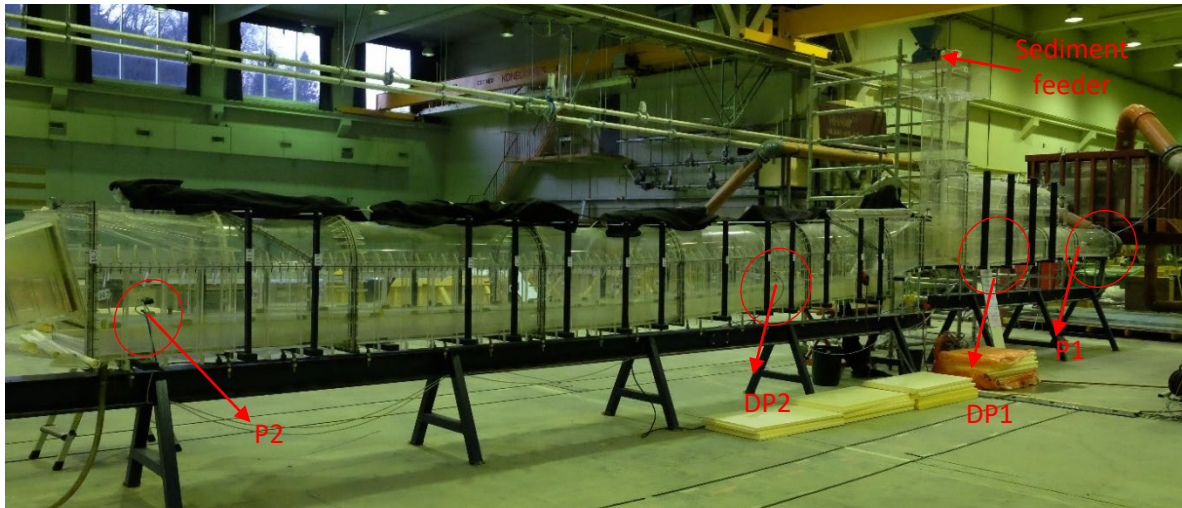
Figure 15: Location of the pressure sensors and differential pressure sensor in the model
