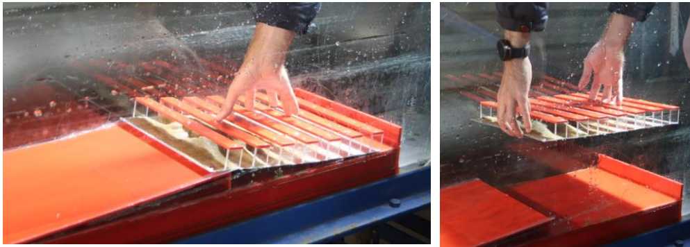
Figure 265: Removable rib construction for sand collection
