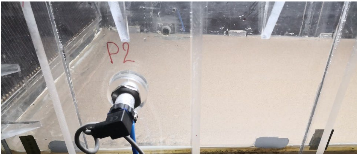
Figure 50: Sediment deposition before the trash rack after modification 2
