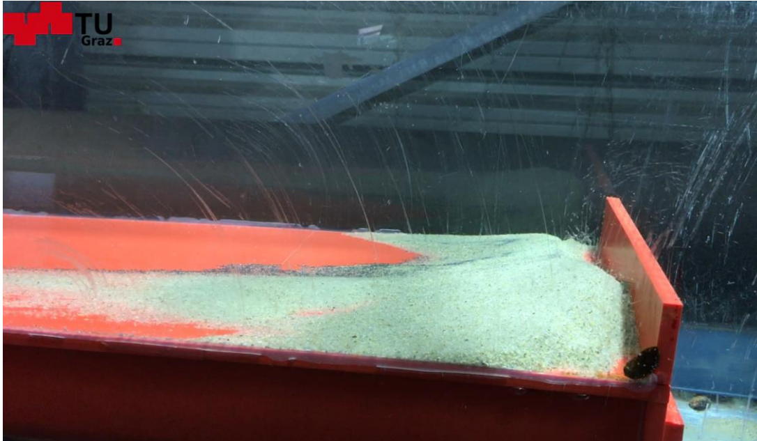
Figure 234: Discharge 41 L/s, sand inflow 0.5 L, sand overtopping weir downstream, snapshot
