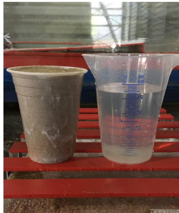
Figure 267: Left; sand input 500 ml, right; measured volume of collected trapped sand in relation to 500 ml input sand
