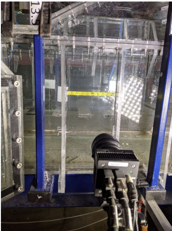
Figure 4 The camera pointing at the ribs. The camera focuses on the calibration object in the middle of the tunnel, therefore the near end of the ribs obstruct the view below the ribs. The flow is from left to right.
