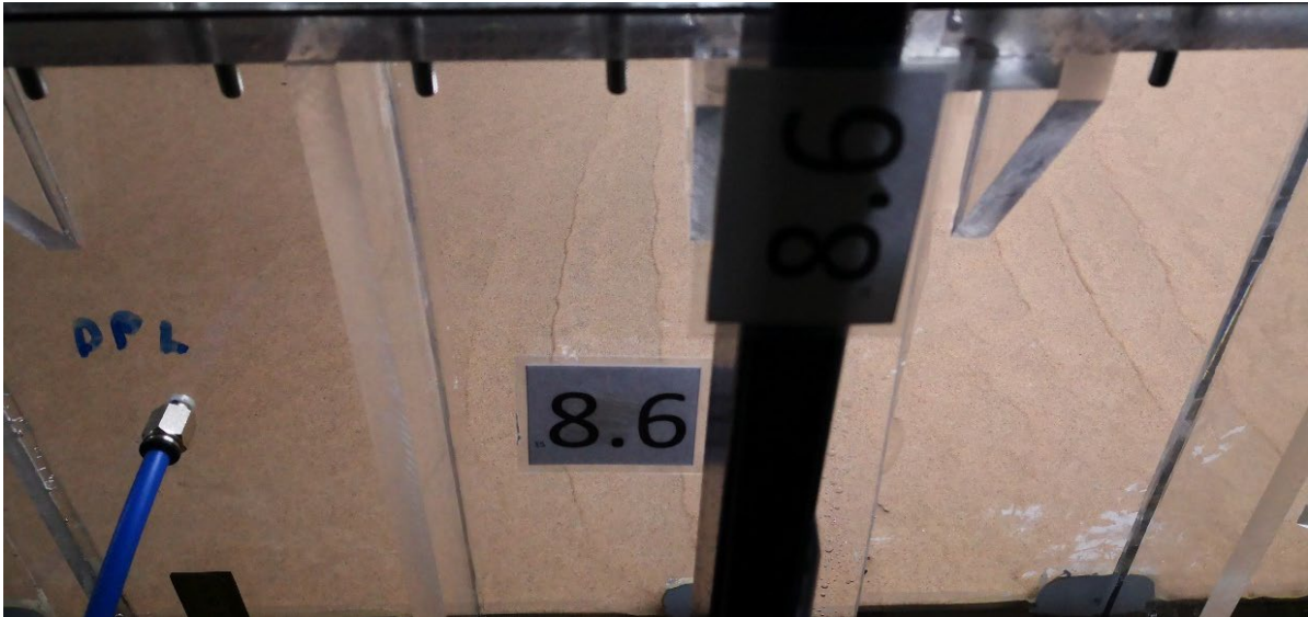
Figure 23: A view of ripples formed at 40 m distance from the start of the sand trap
