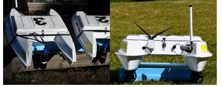
Fig. 3. The ASVs used in the experiments. The left and right pictures show the front and back of the "ducklings" where the acoustic receivers and thrusters, RFD868 and Wifi antennas can be seen, respectively.
