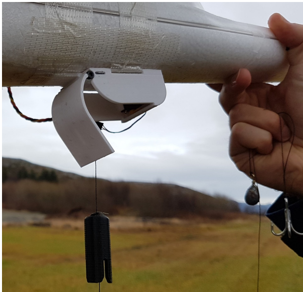
Fig. 7: The pod used to hold the hook and catch line. The pod is mounted on the fixed-wing airframe with glass fibre reinforced tape. On the line hanging from the pod is a cylinder used to wind the catch line up on. The hook and weight (shown to the right in the hand) is put inside the cylinder when the line is wound up.
