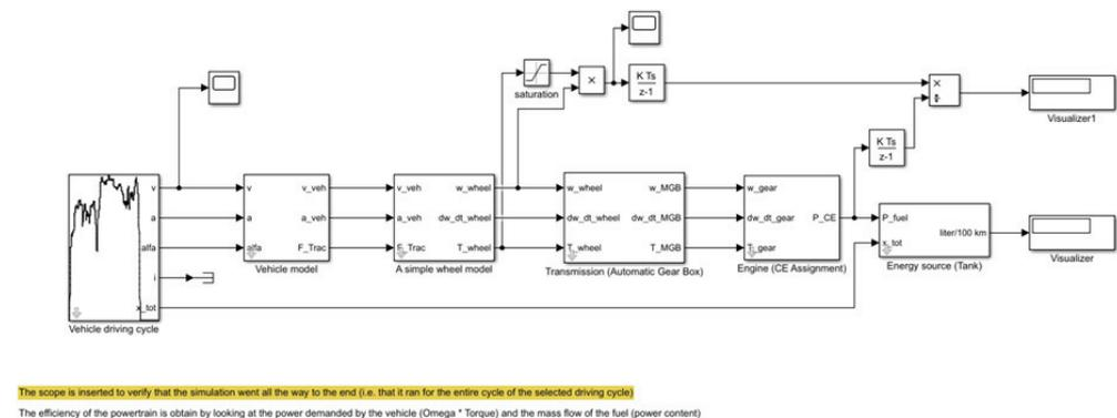
Figure 1. QSS model of the conventional truck (12 tons GVW)
