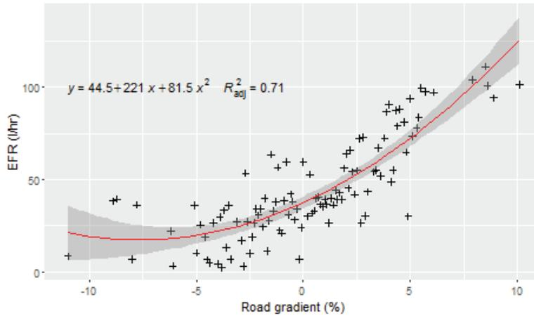
Figure 5.2 eco-driven HDV Engine fuel rate (EFR) vs road gradient. This is a second order (polynomial) model
