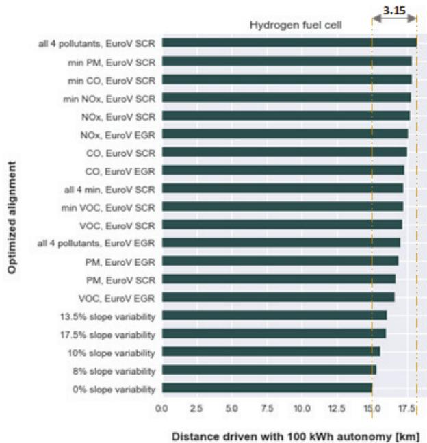
Figure 5.18 Efficacy of a 12-tons hydrogen fuel cell electric truck
