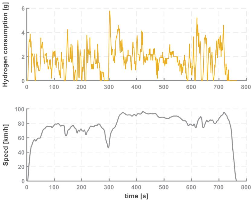
Figure 13. Hydrogen consumption of the designed fuel cell truck.
