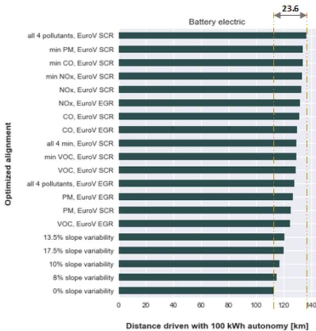
Figure 5.20 Efficacy of a 12-tons battery electric truck
