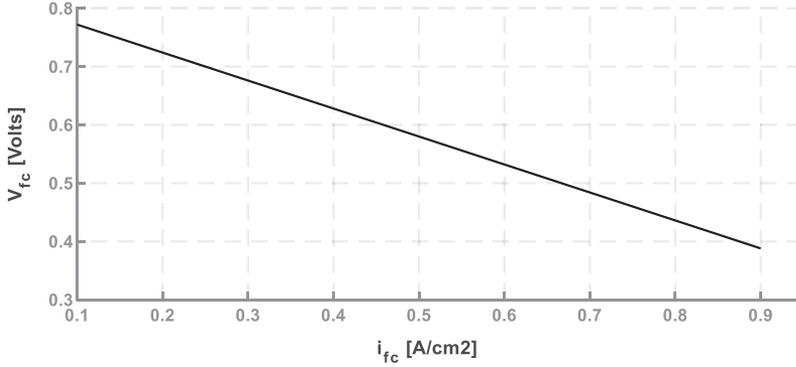
Figure 11. Polarization curve of a typical cell.
