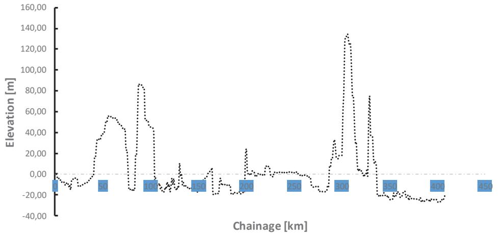
Figure 4.3 Profile of the vertical alignment of the retained portion of the Norwegian coastal highway E39.
