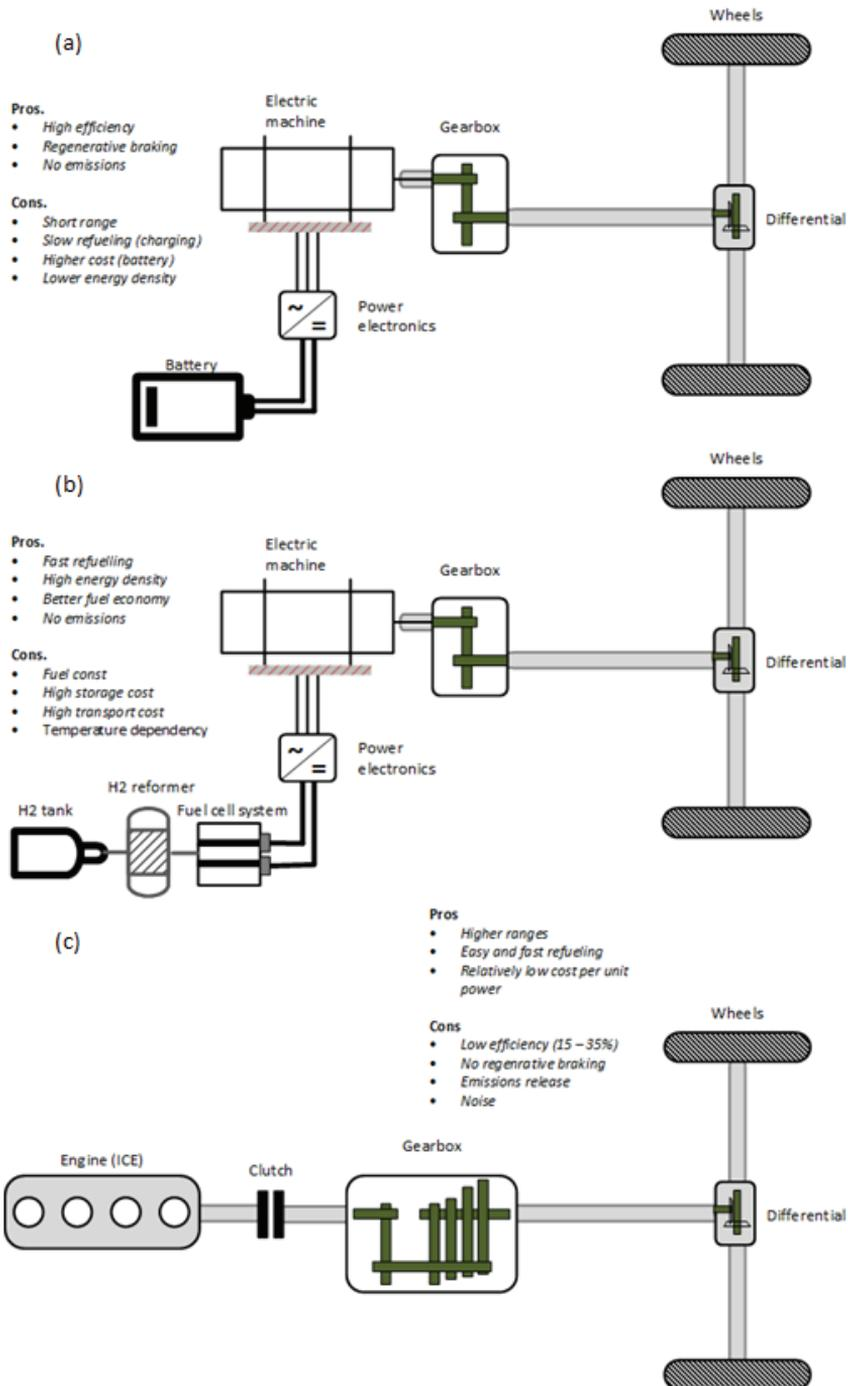
Figure 3.4 High-level configurations of the studied powertrains
