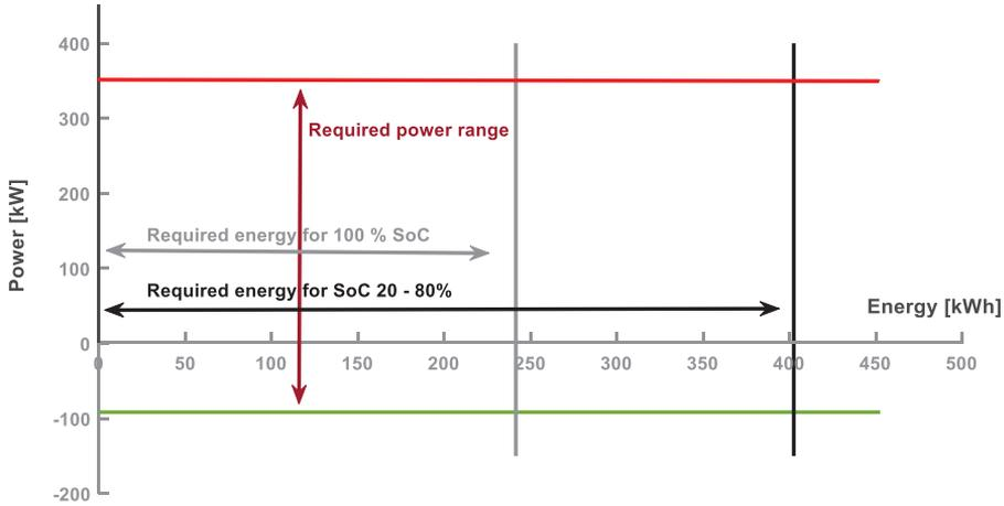
Figure 10. The operational range of the sized battery pack.
