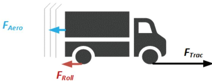
Figure 3. A simplified representation of vehicle forces.
