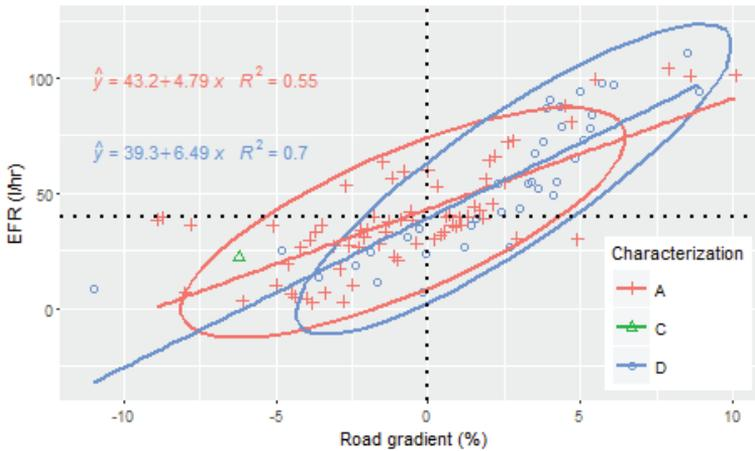
Figure 5.3 eco-driven HDV, multi-mode Engine fuel rate (EFR) vs road gradient. First order (linear) models. Blue: acceleration, Green: constant speed, Red: deceleration.
