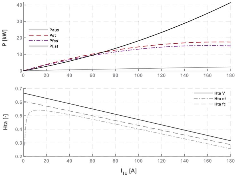
Figure 12. Power and efficiency profiles of a typical fuel cell system.
