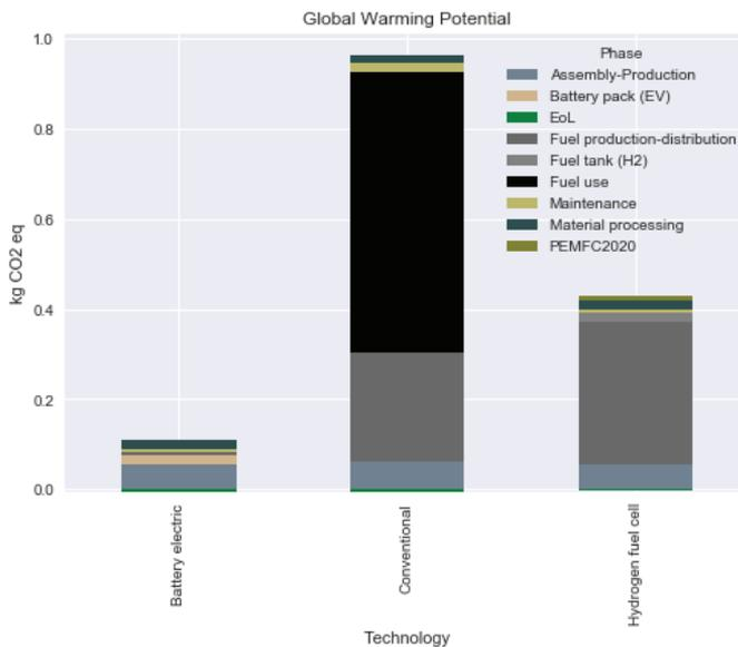
Figure 5.10 Global warming potential of the three trucks on best-case alignment
