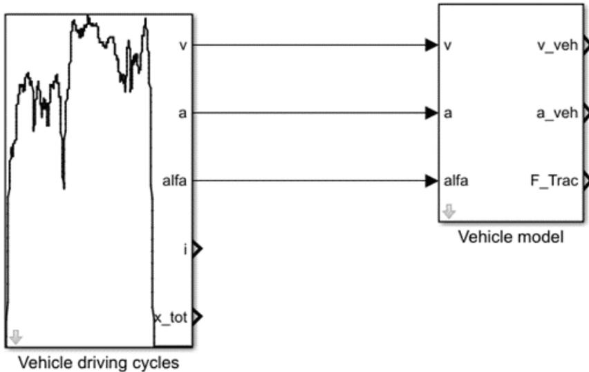
Figure 2. The two stage of QSS model used in the design of clean trucks (i.e. battery electric and fuel cell electric trucks, 12 tons GVW)
