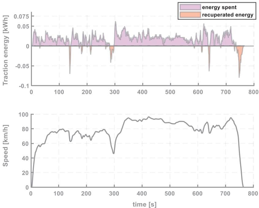
Figure 9. Profile of traction and recuperated energy of the designed trucks.
