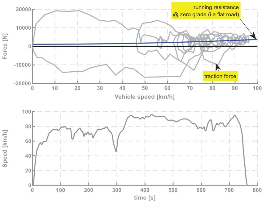
Figure 5. Traction force of the designed trucks.
