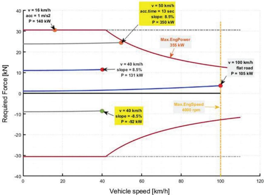
Figure 8. Operating points of the designed trucks.
