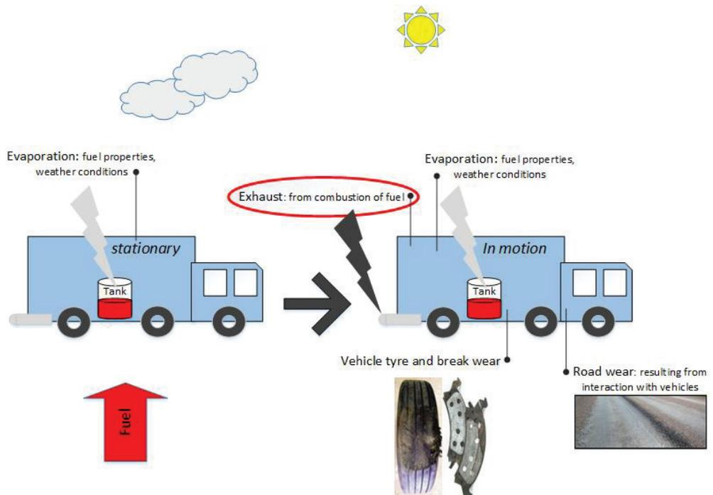
Figure 2.1 Simplified representation of road vehicle's emissions flows
