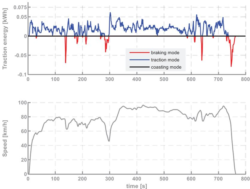
Figure 7. Mode-related traction energy of the designed trucks.
