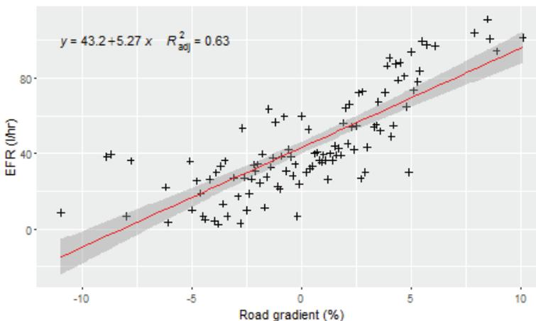
Figure 5.1 eco-driven HDV Engine fuel rate (EFR) vs road gradient. This is a first order (linear) model
