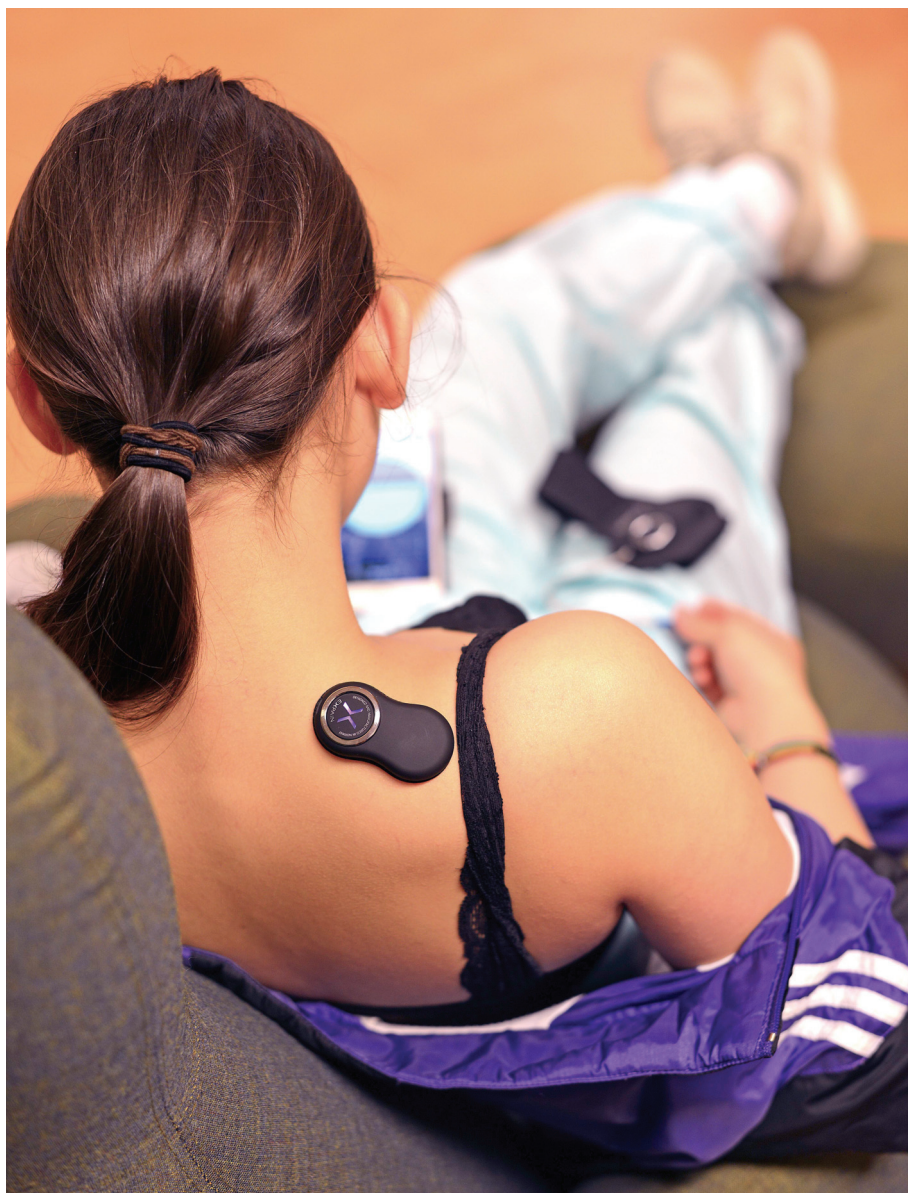
Photo 1: The muscle tension sensor in use. Placed over the upper trapezius muscle fibers midway between the acromion and spinous process of C7 and attached to the skin by a sticky electrode with conductive gel.
