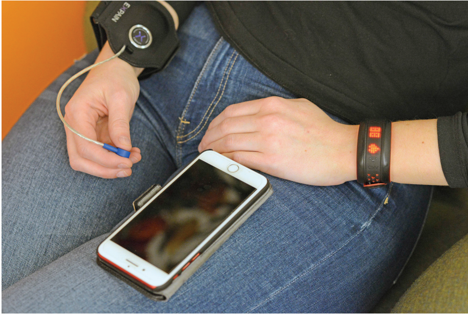
Photo 3: The temperature sensor and the heart rate wristband in use. The thermistor is held between the thumb and index finger of the right hand. The heart rate wristband sensor is worn as a watch around the left wrist and measures heart rate on the dorsal aspect of the forearm.
