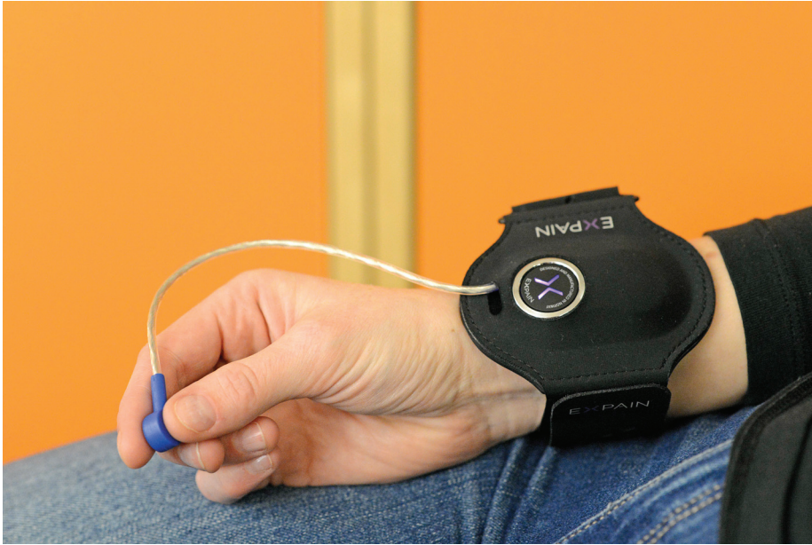
Photo 2: The temperature sensor in use. The thermistor is held between the thumb and index finger of the right hand. The thermistor is soldered onto a NeckSensor™, to use this for signal processing and Bluetooth® transmission.
