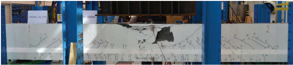
Figure 2— Final failure state of beam 4
