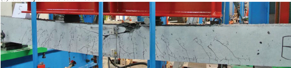
Figure 4 – Final failure state for beams (a) 2.3-1; (b) 2.3-2; (c) 4.0-3; (d) 4.0-4 and (e) 3.43-5
