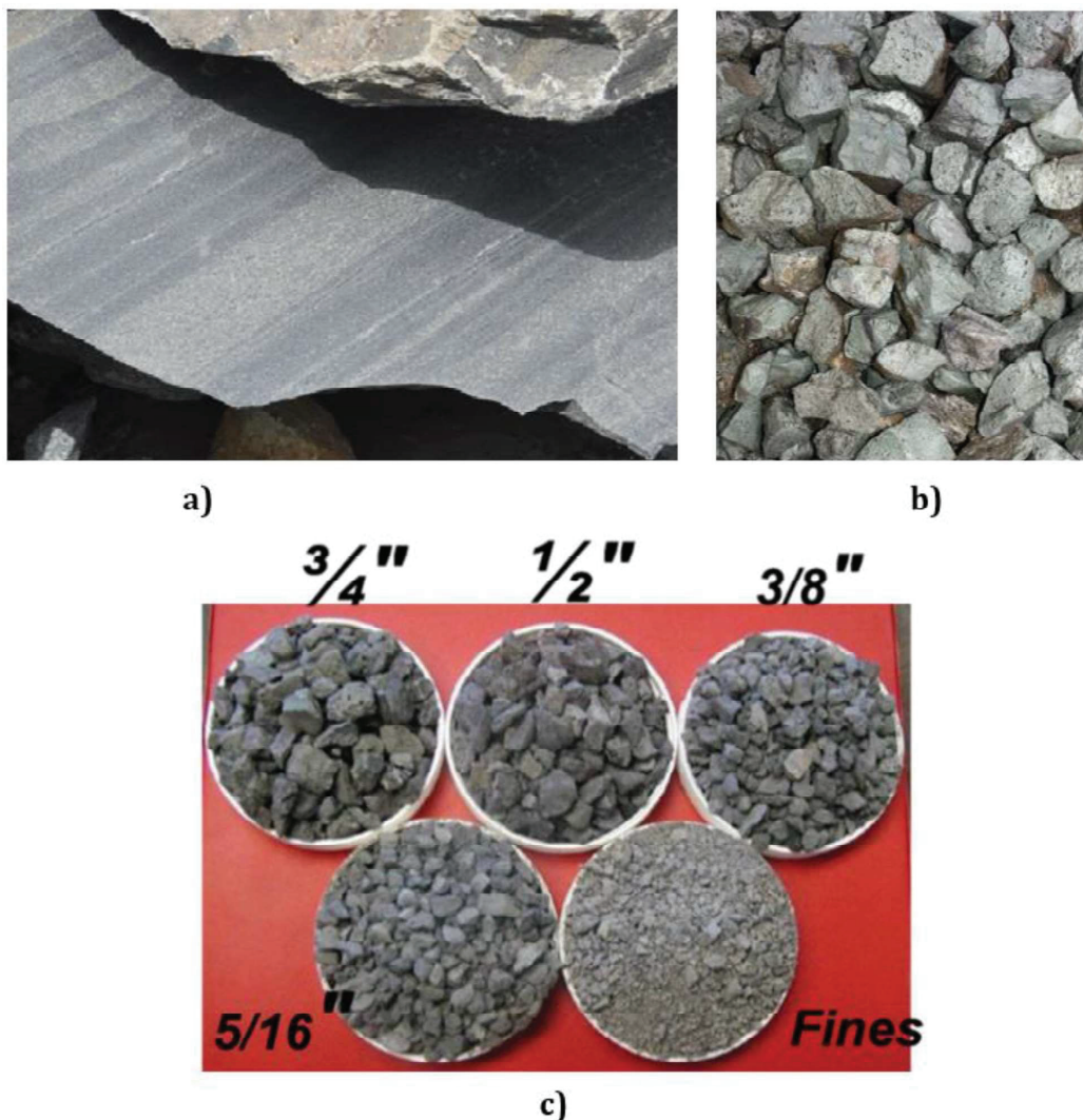
Figure 1: a) Stone of argillite slate; b) LWA Stalite; and c) Fractions of Stalite material [ Stalite Structural, 2020 ].
