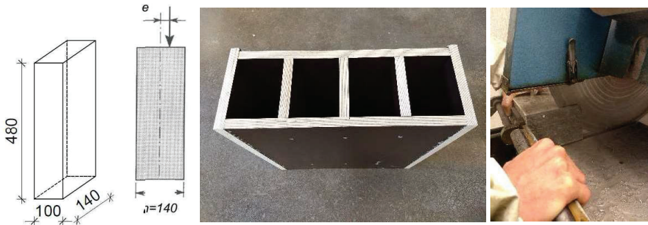
Figure 1 – Geometry of the prisms (left), Forms for the prisms (centre), Preparation of the prisms (right).
