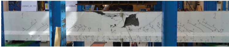
Fig. 4 Figure of the failure for beam 4 (LWAC65_20_100).
