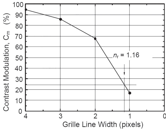
FIGURE 3 Contrast modulation example as shown in the Information Display Measurements Standard (IDMS) standard. Measurements are done with Grilles of 1, 2, 3 and 4 pixels width, while linear interpolation makes up the intermediate values
